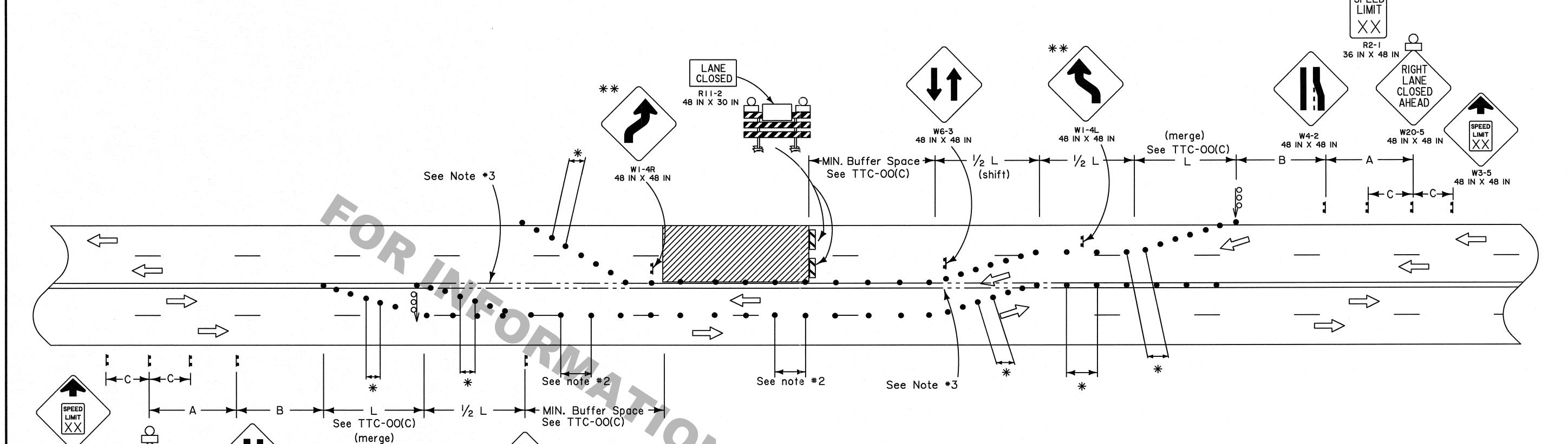
\* See TTC-00(C) for spacing of channelizing devices in tapers and tangent areas.
