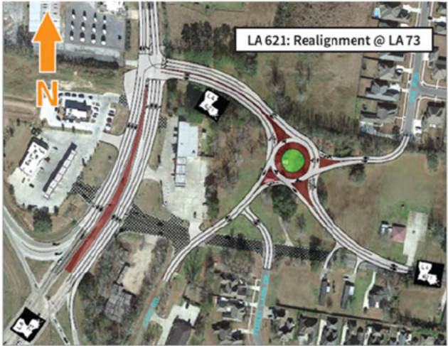
This is the conceptual layout completed by NSI prior to preliminary plans to provide DOTD with the potential impacts and proposed geometry before producing 30% preliminary design plans.
