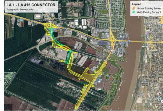
traffic segments of LA 1, Interstate 10 ramps, and LA 415. The data was processed through Trimble Business Center, with data extraction performed through TopoDot. The survey is being conducted according to the Louisiana Department of Transportation and Development Location and Survey Manual. The deliverables will be provided in accordance with the LADOTD guidelines for electronic deliverables.
