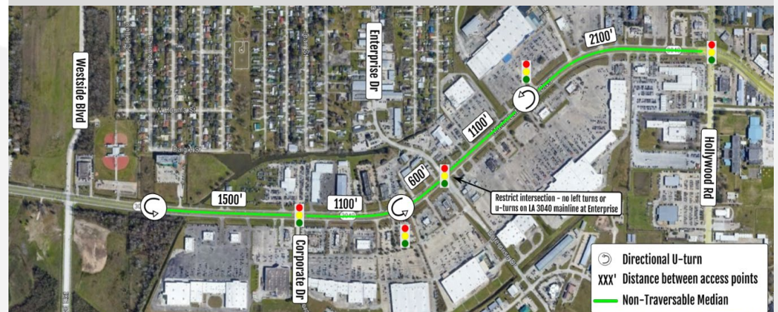
Figure: Build concept showing raised median with formalized u-turn location to reduce conflict points.
