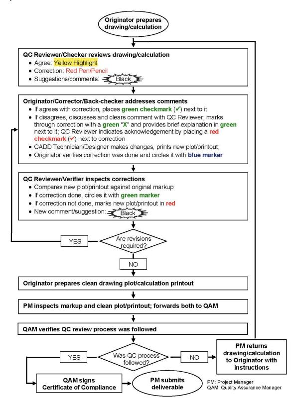
Figure 5: Drawing and Calculations Quality Control and Quality Assurance Process
