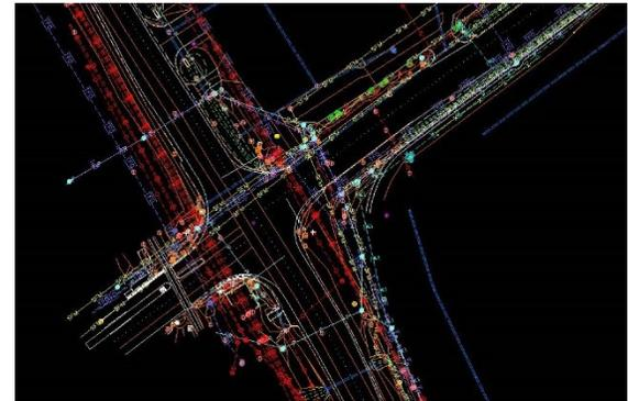
Figures: Topographic Survey of the Nicholson/Gardere Intersection and Property Survey Deliverable for Staring Lane Extension
