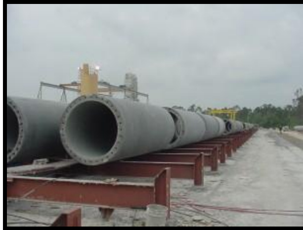
Segments of Precast Cylinder Piles before Post Tensioning
