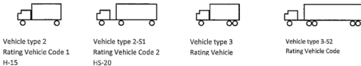
FIGURE 4. TIMBER BRIDGES ASR METHOD RATING VEHICLES
