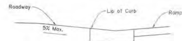
TRANSITION FROM CURB RAMP TO ROADWAY
