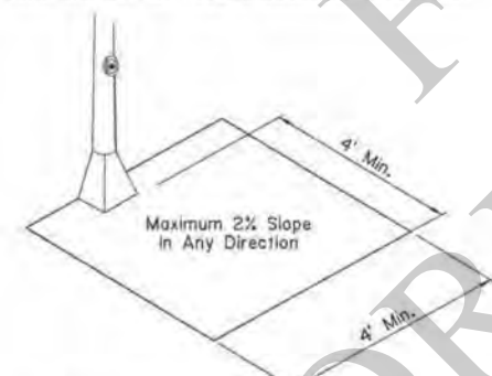
CLEAR GROUND SPACE ADJACENT TO PEDESTRIAN PUSH BUTTON Minimum 4' x 4' clear space required at public use fixtures.
