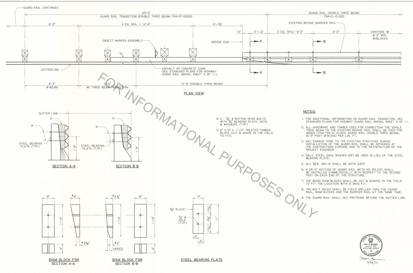
\* DIMENSIONS ARE ASSUMED. ADJUST IN THE FIELD AS REQUIRED. HOLES SHALL BE DRILLED IN THE FIELD. SEE NOTE NO. 8.
