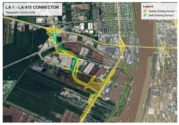
and LA 415. The data was processed through Trimble Business Center, with data extraction performed through TopoDot. The survey is being conducted according to the Louisiana Department of Transportation and Development Location and Survey Manual. The deliverables were provided in accordance with the LA DOTD guidelines for electronic deliverables.
