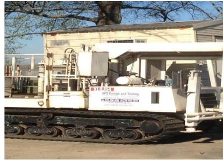
14-Ton track-mounted Cone Penetrometer System
