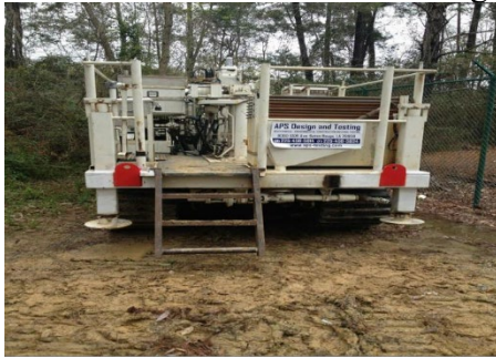
14-Ton track-mounted Cone Penetrometer System
