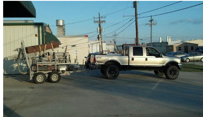
Simco 4000 on trailer-Drill depths 80 feet
