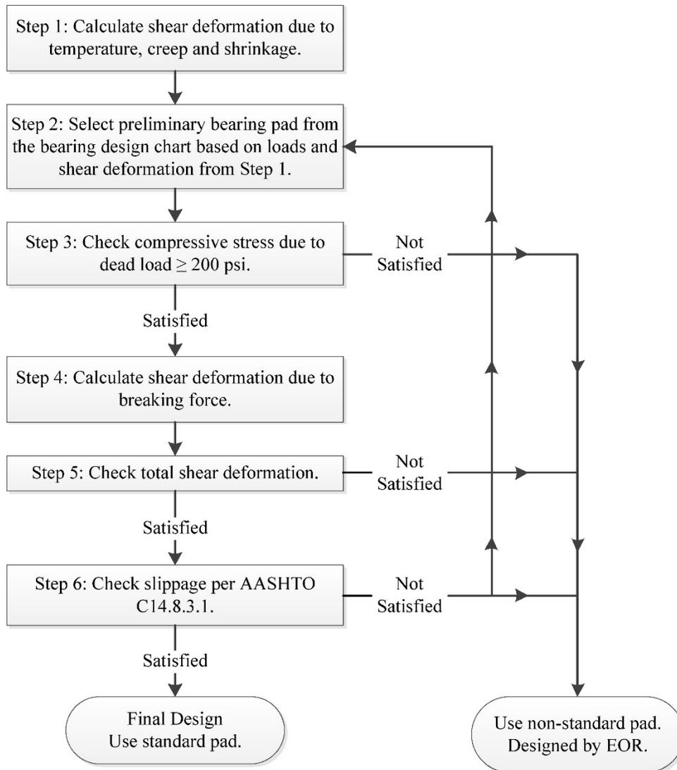
**Figure 1.2.3-1: Flowchart to Use the Bearing Design Chart**
