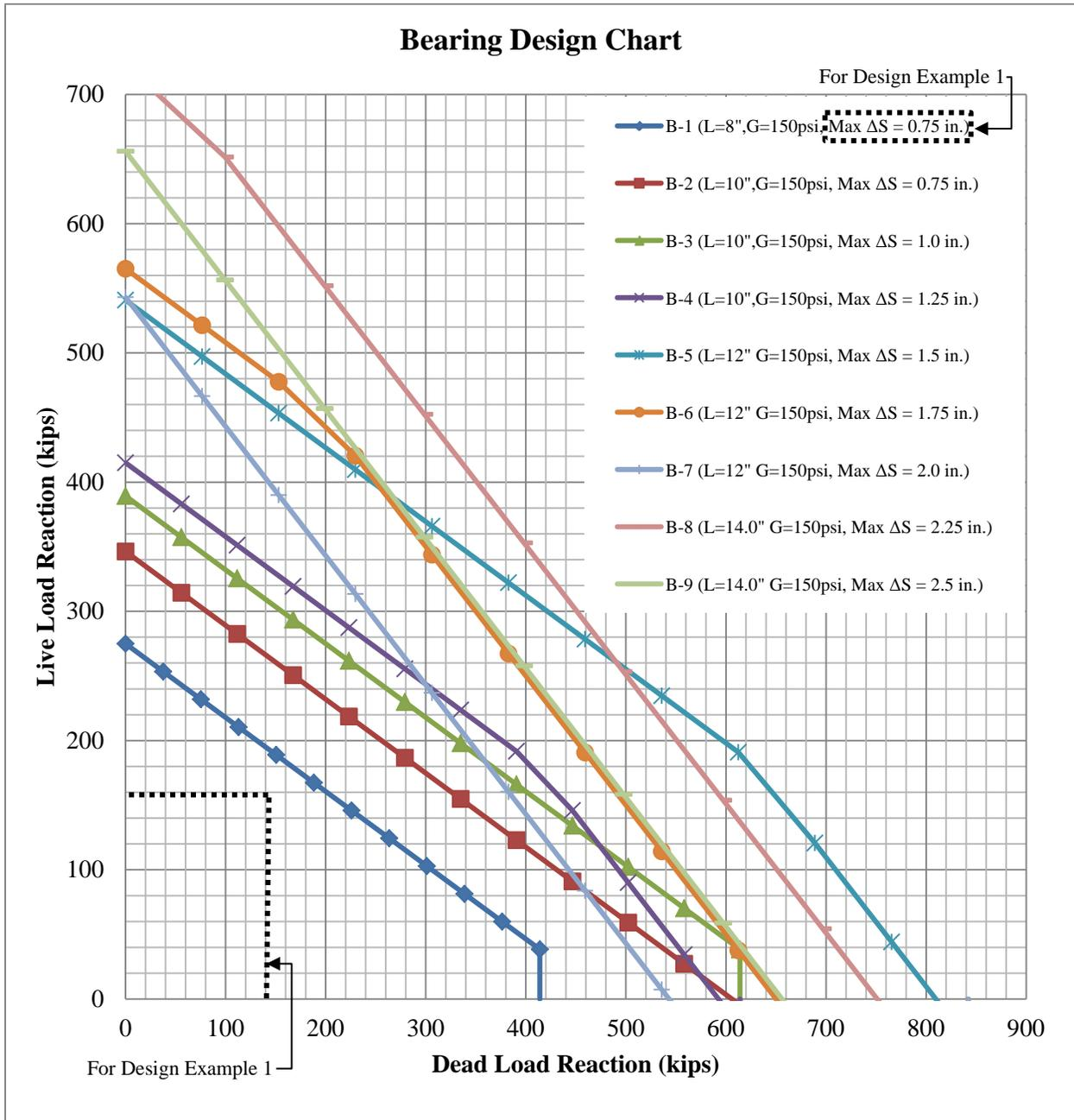
**Figure 1.2.4.1-2: Bearing Design Chart - Example 1**
