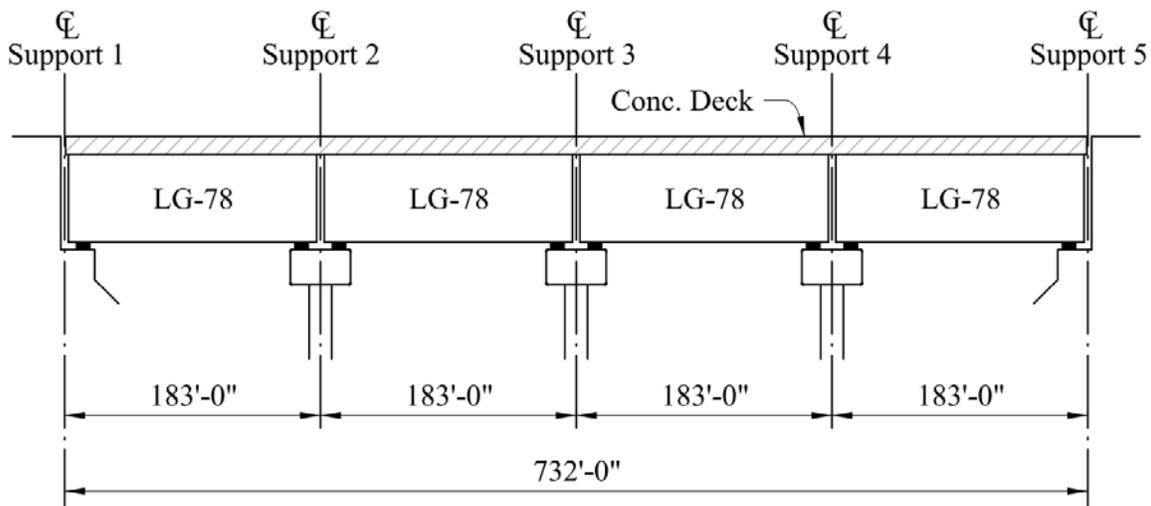
**Figure 1.2.3.2-1: Bridge Profile for Design Example 2**
