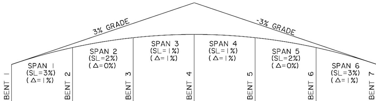
In this example, the slope of the girders (SL) is shown. Assuming that the bearing pads are all the same size, then the beveled plates at the girder ends shall all be specified with a 2% slope.
