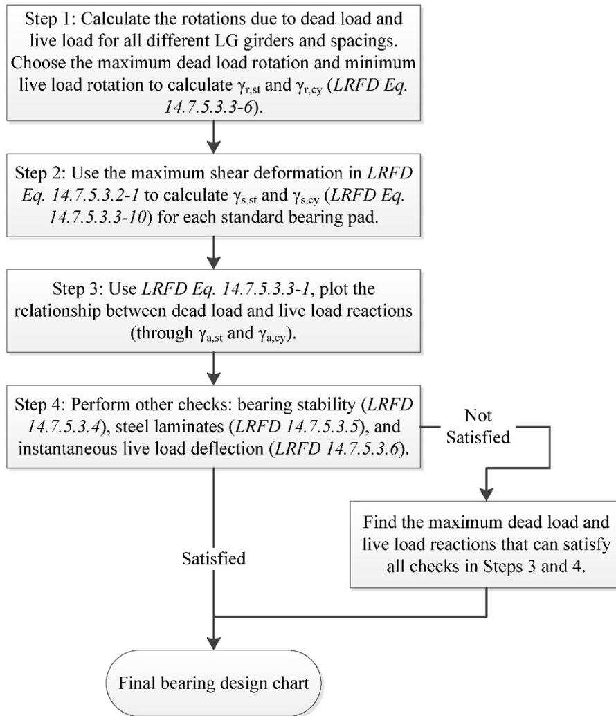
**Figure 1.2.2-1: Flowchart for Developing Bearing Design Chart**
