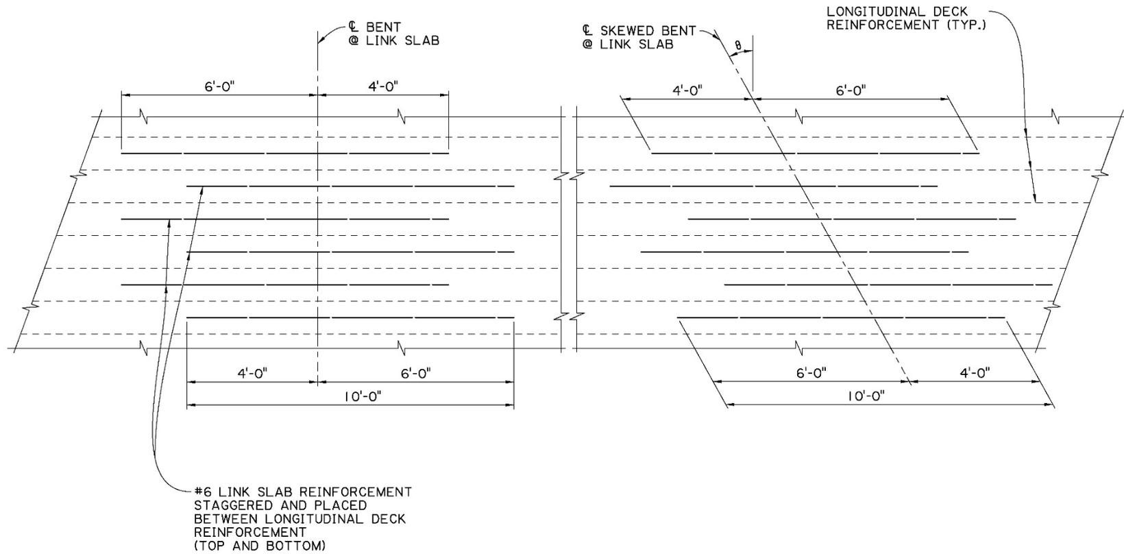
LINK SLAB REINFORCEMENT
