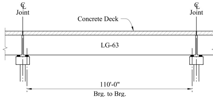
**Figure 1.2.4.1-1: Bridge Profile for Design Example 1**
