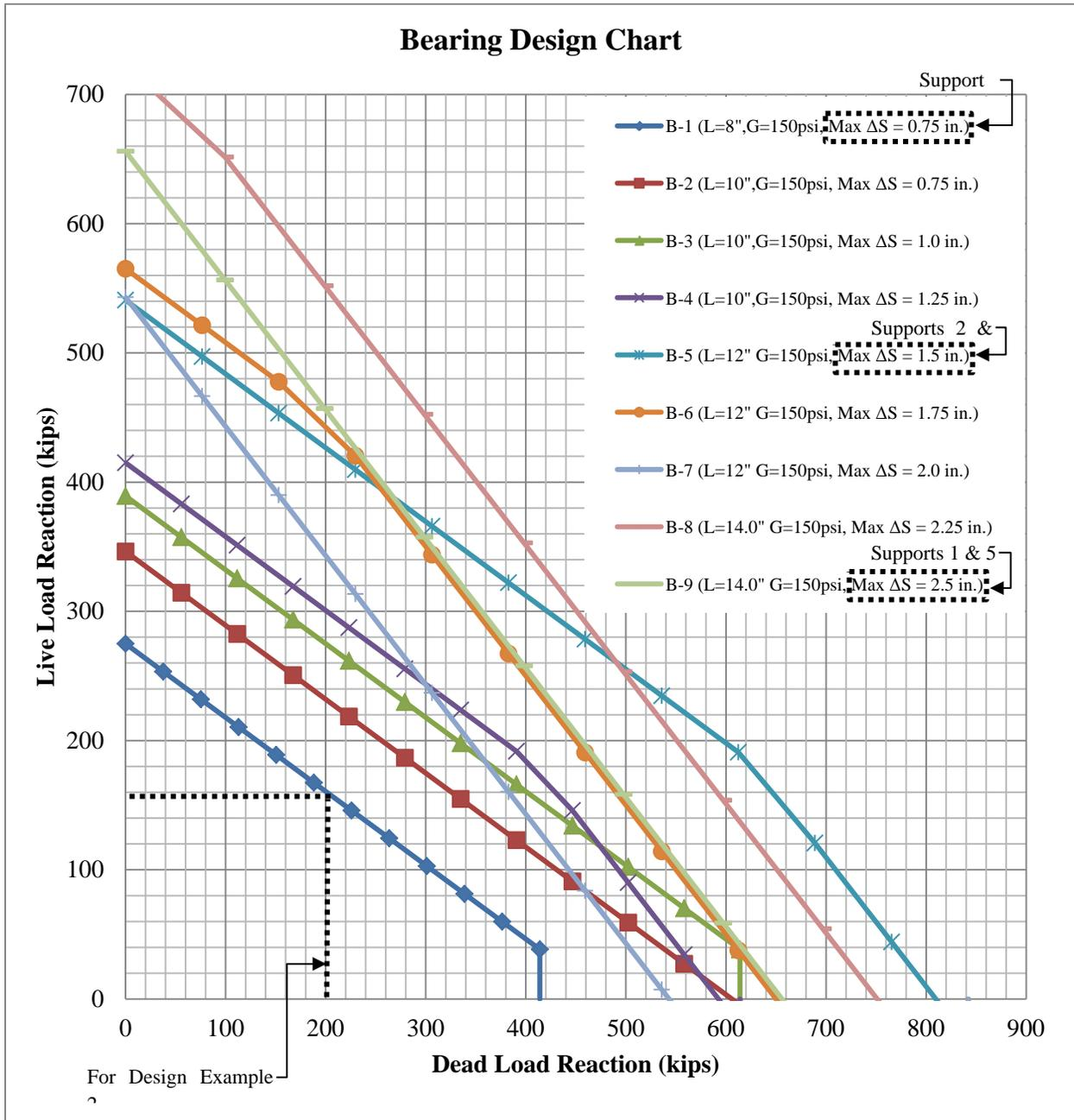
**Figure 1.2.4.2-2: Bearing Design Chart - Example 2**
