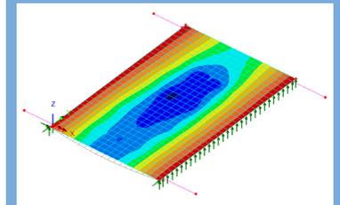
F&T used a LUSAS FE Model to remove the posting on a slab span bridge after the typical AASHTOWare BrR method resulted in a load posting.
