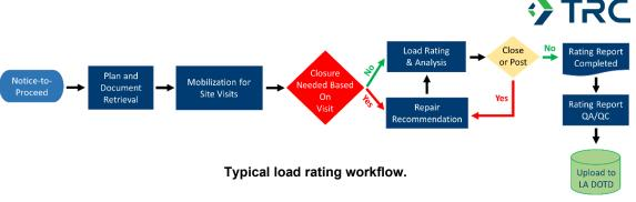
storm events and provide critical findings during a scheduled routine or special inspection. If a bridge is recommended for closure, TRC will provide recommendations as part of the load rating reports (where appropriate) for immediate repair(s) to keep the bridge open to traffic.
