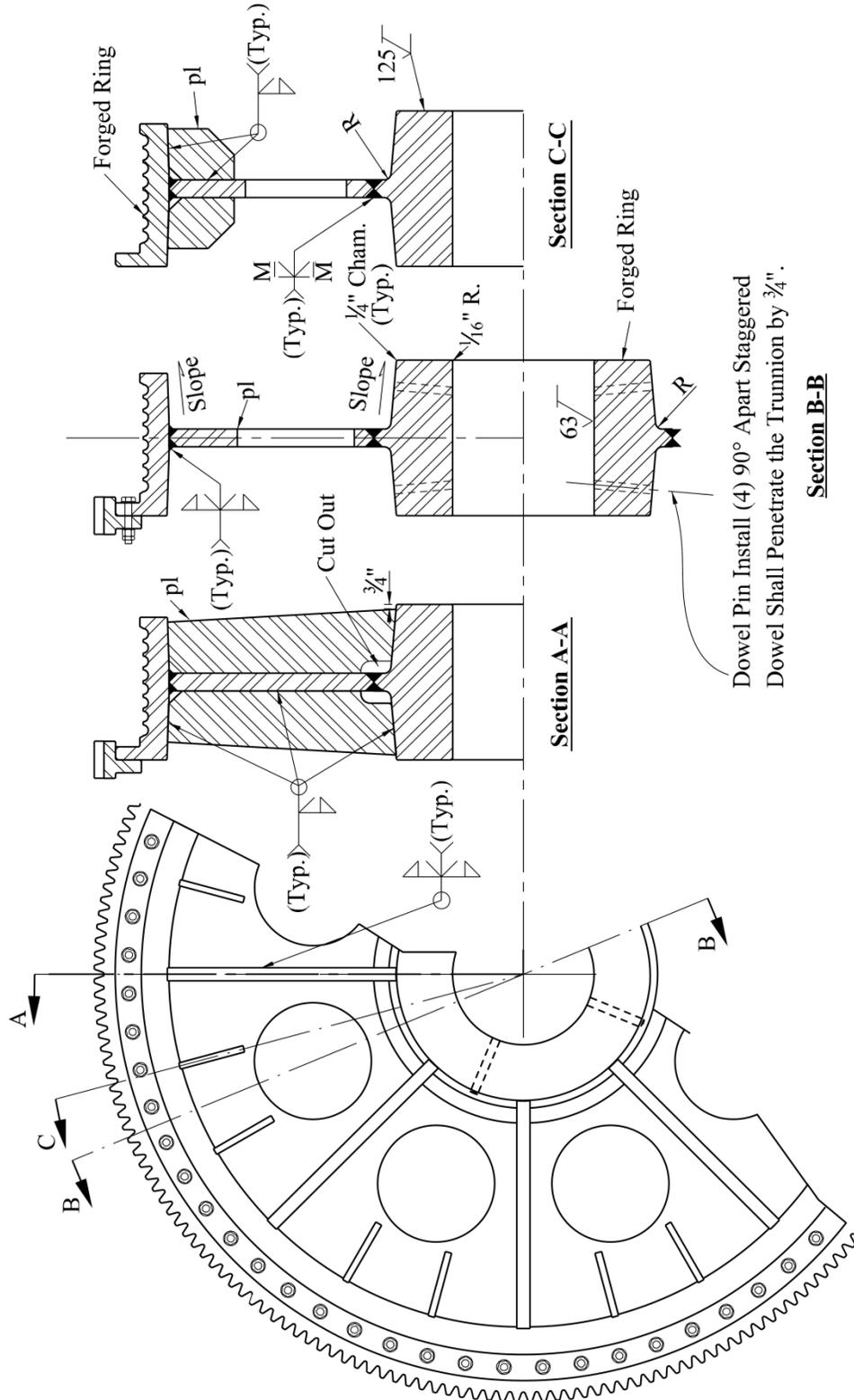
**Figure 6.8.3.4.2-1—Single Web Counterweight Sheave**
