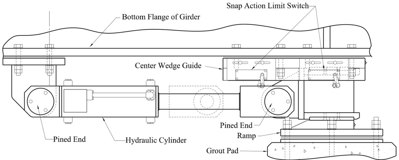
Figure 6.8.2.5-1—Typical Center Wedge Assembly
