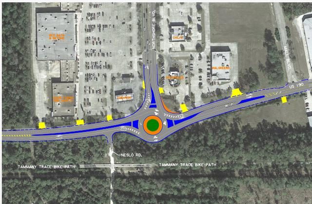
T. Baker Smith served as the prime consultant on the project providing all roadway design, hydraulic analysis, preliminary and final plan development, a specialized and detailed written construction phasing plan as well as oversight of temporary traffic signalization design for use during construction. TBS has submitted 98% Final Plans to LADOTD in December 2022. LADOTD subsequently placed the project on hold due to funding. TBS expects to submit 100% Final Plans once project resumes.
