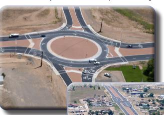
**Project Description** The project involved the design of improvements to reconstruct an existing 3-mile section of 2-lane SR 89 to a 4-lane roadway with a 20-foot raised median. The project included the design of a roundabout at a major intersection at Road 4 South to optimize traffic demands and future vehicular movements.
