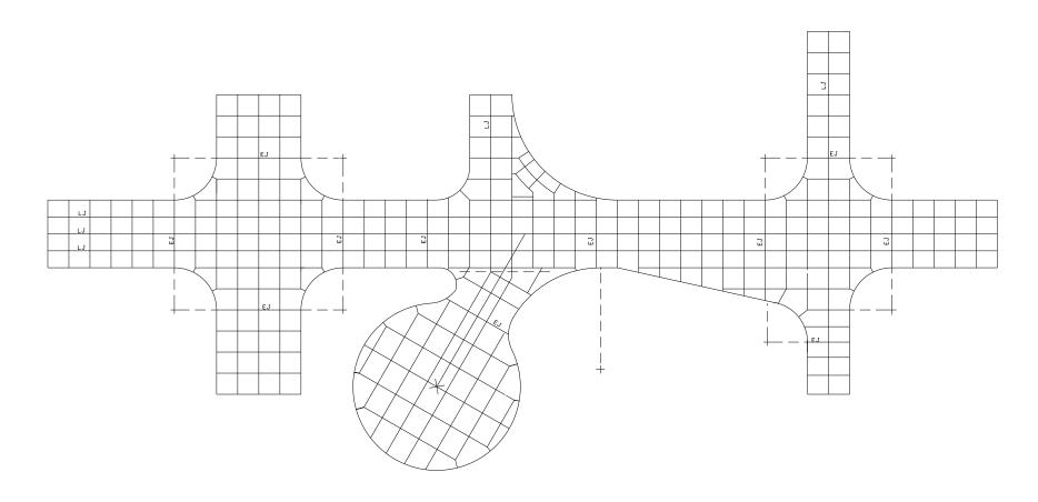
Note: All Joints are Dummy Joints Unless Specified otherwise.(See Also Standard Plan CP-01)
