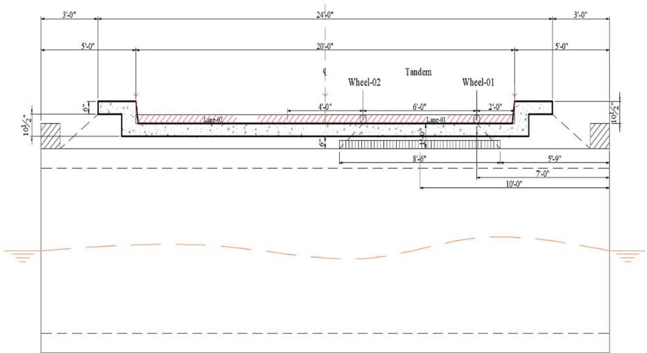
Live load distribution at the surface of the top slab in the direction perpendicular to the culvert span for fill height of 1.0 ft
