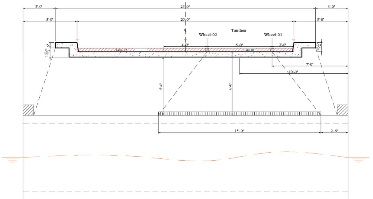
Live load distribution at the surface of the top slab in the direction perpendicular to the culvert span for fill height of 6.0 ft
