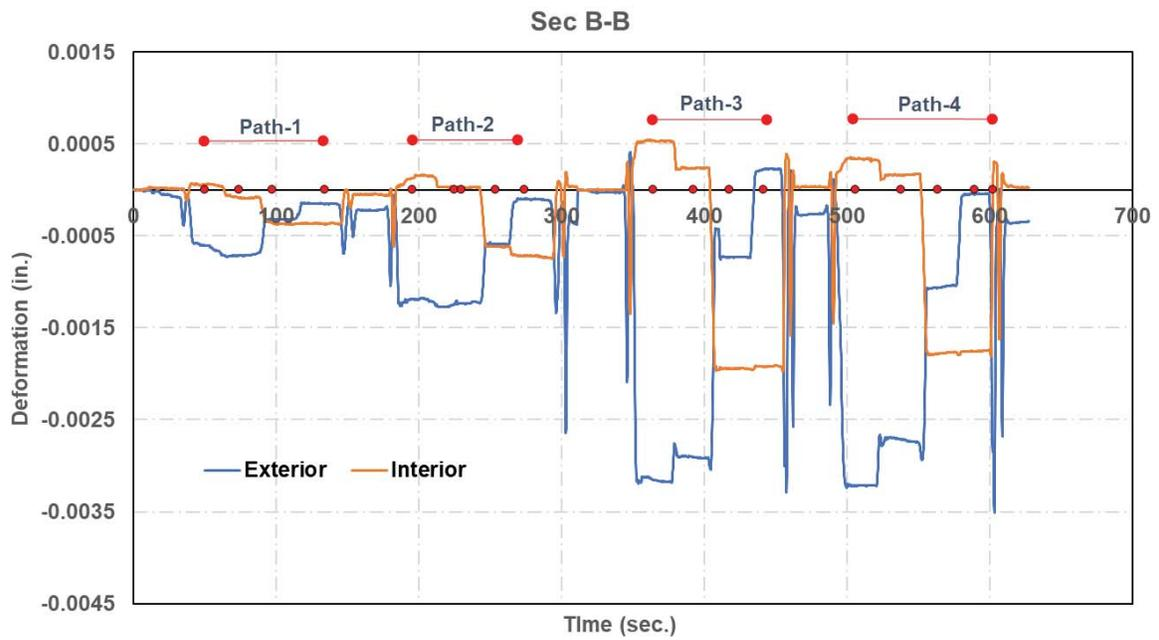
Vertical displacement at mid span of Exterior and Interior Cells for Load Path 1 and Load Path 2
