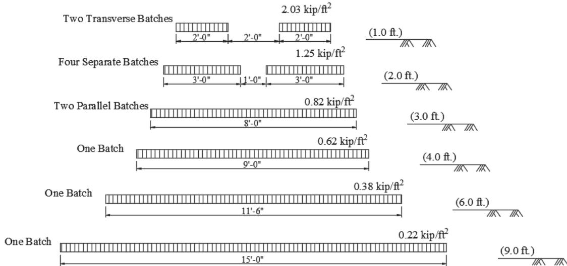
Live load distribution at the surface of the top slab in the direction parallel to span for 12 x 12 culverts
