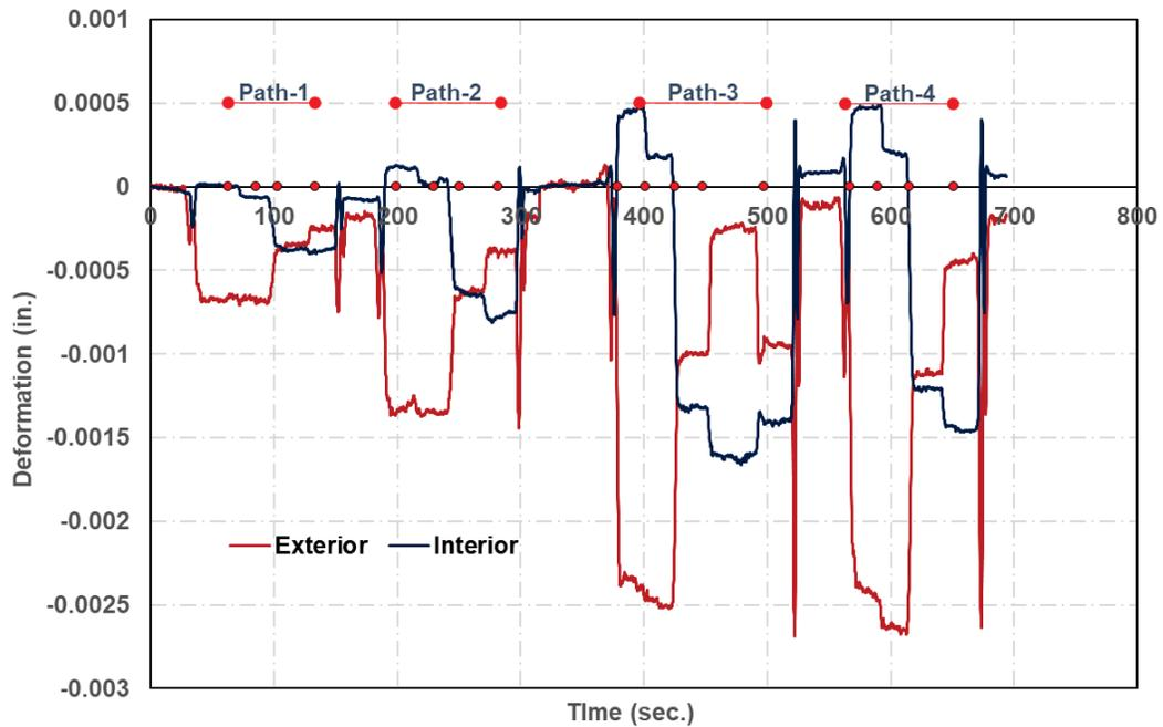
Vertical displacements at midspan of exterior and interior cells during loading of Culvert
