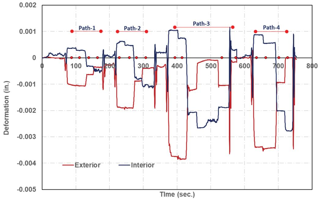
Vertical displacement at midspan of exterior and interior cells during loading
