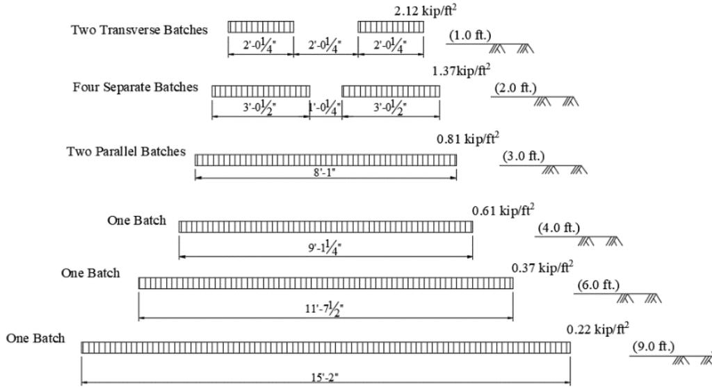
Live load distribution at the surface of the top slab in the direction parallel to span for 7 x 7 culverts
