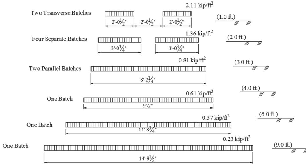
Live load distribution at the surface of the top slab in the direction parallel to span for 8 x 8 culverts
