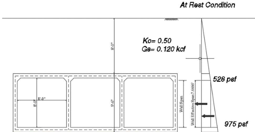
Figure 7: At rest lateral soil pressure linear distribution on the exterior wall of a culvert with 8.0 ft fill height
