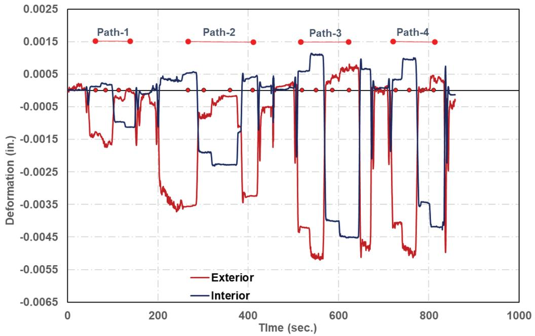
Vertical displacement at midspan of exterior and interior cells during loading of Culvert
