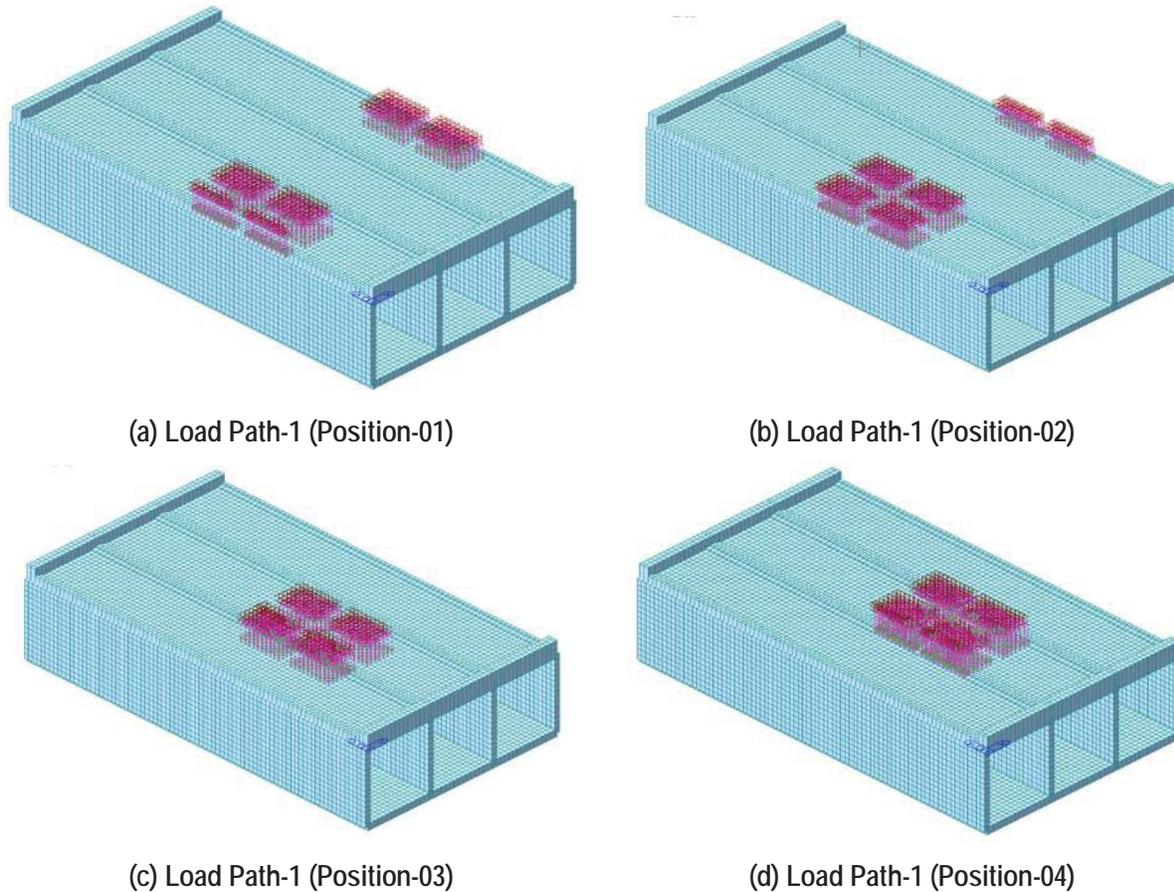
Figure 49: Truck load positions for load path 1
