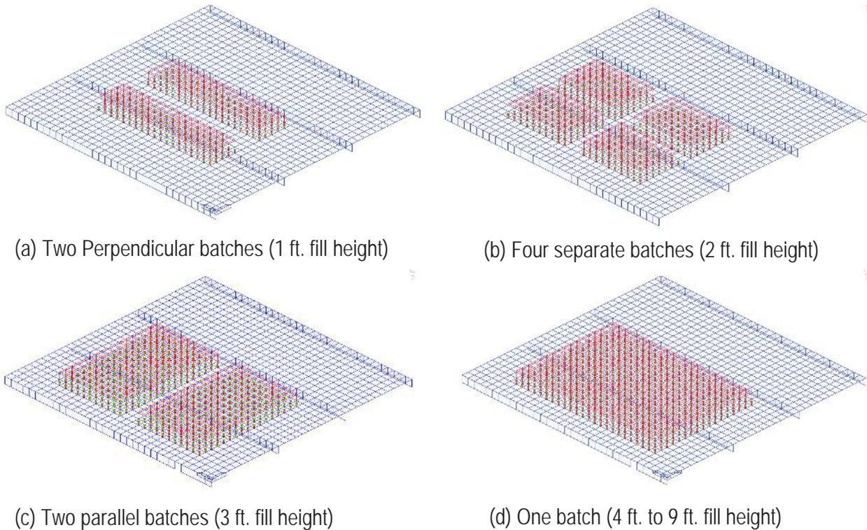
**Figure 31: Live load configurations at the surface of the top slab**
