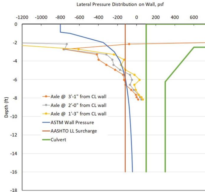
Figure 11: Live load surcharge pressure on culvert wall against backfill depth (adopted from NCHRP 15-54)
