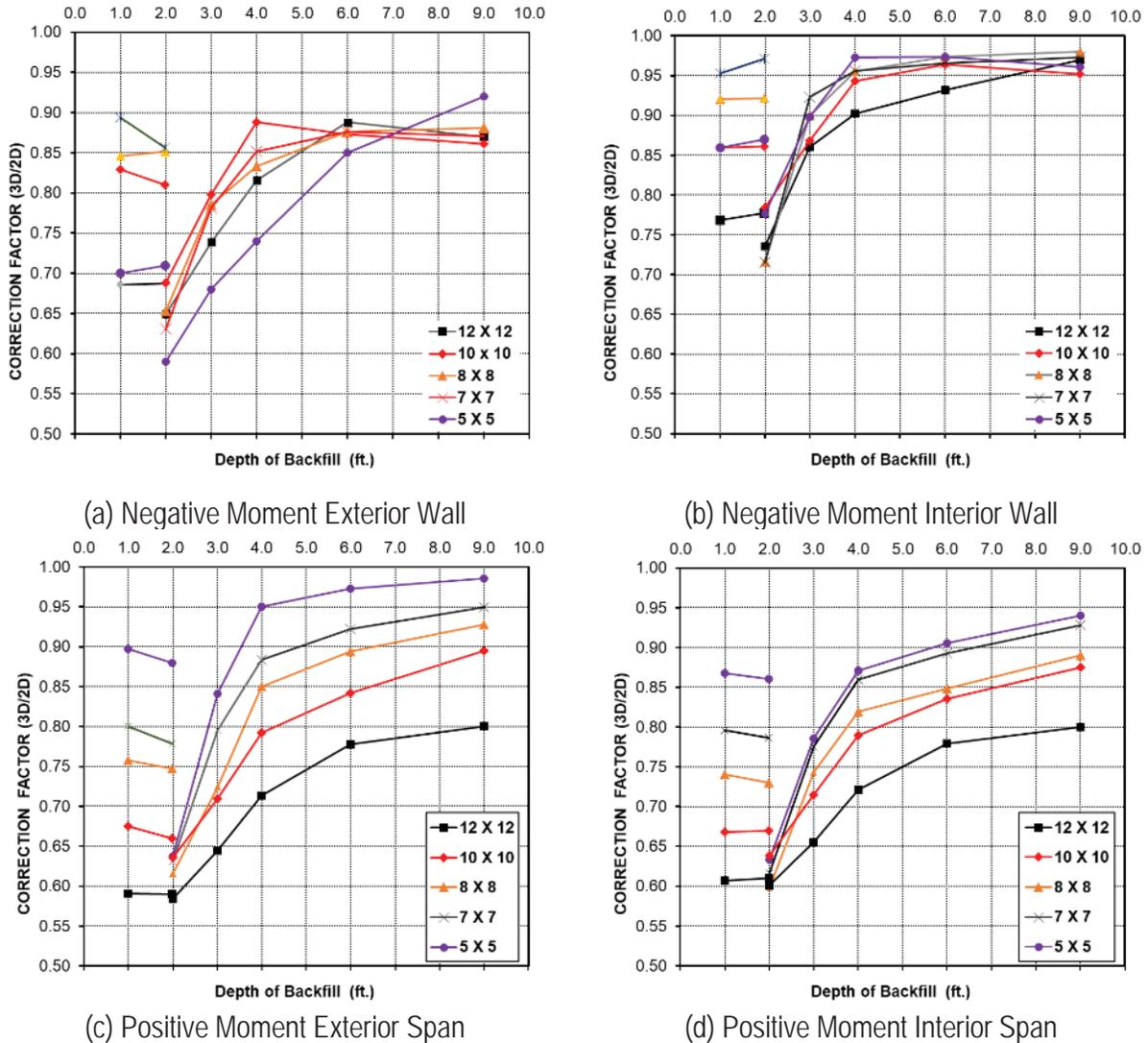
Figure 40: Correction factors between 2D and 3D models for culvert with different sizes
