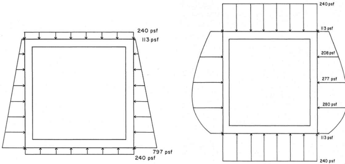
Figure 6: (a) at rest linear distribution for the lateral soil pressure (AASHTO) on culvert exterior wall and (b) measured nonlinear distribution for the lateral soil pressure due to soil arching effects.
