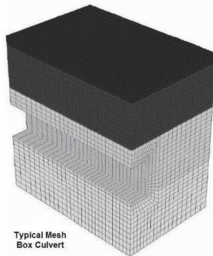
**Figure 18: Three-dimensional finite element mesh of soil-structure model of box culvert**
