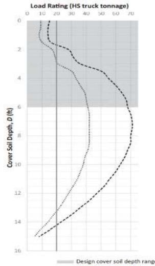
Figure 12: Effect of fill height on the load rating (adopted from Wood et al., 2015)
