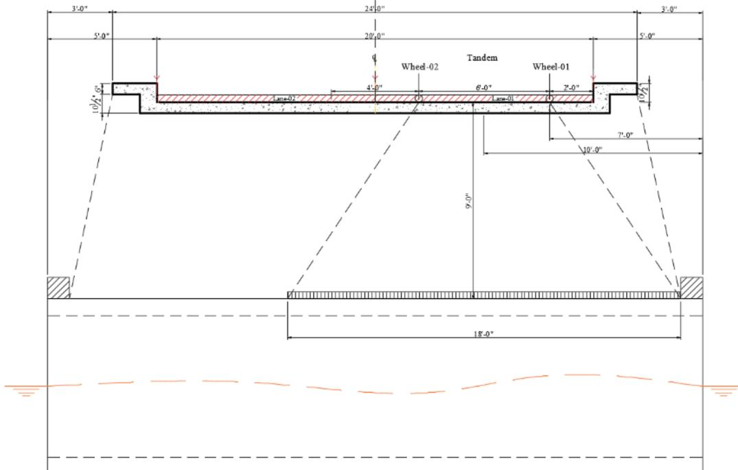
Figure 33: Truck positioning in the direction perpendicular to culvert span
