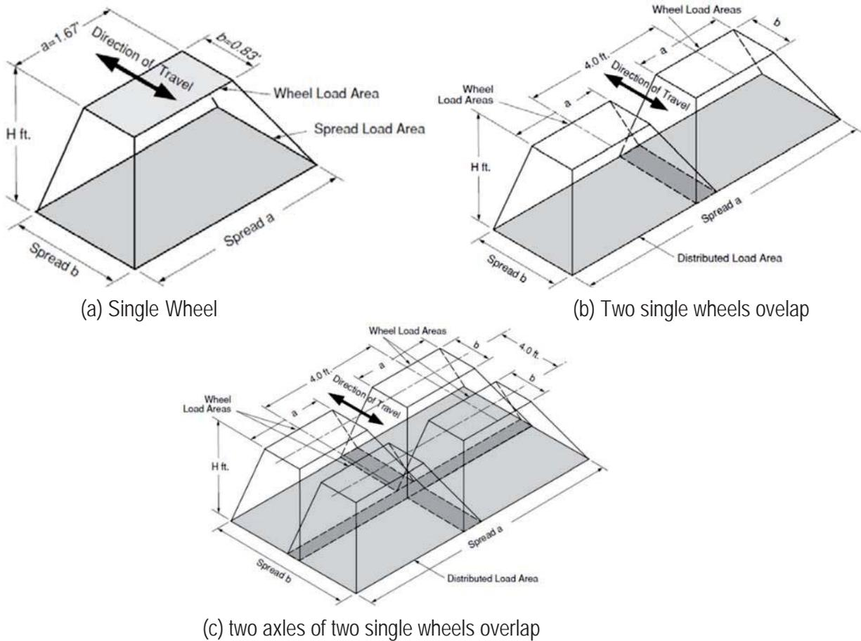
Figure 10: Area of live load distribution for different wheel configuration (Okeil et al., 2018)
