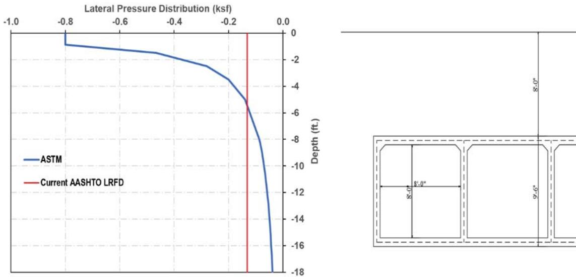
Figure 63: Live load surcharge from ASTM standards versus AASHTO LRFD
