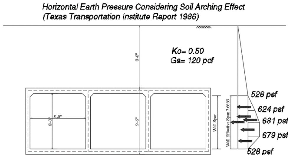
Figure 8: lateral soil pressure including soil arching effects on the exterior wall of a culvert with 8.0 ft fill height
