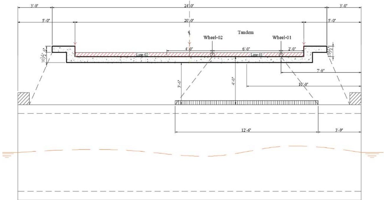
Live load distribution at the surface of the top slab in the direction perpendicular to the culvert span for fill height of 4.0 ft
