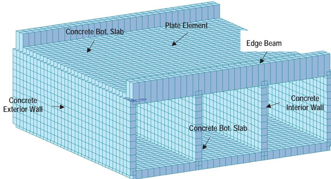
Figure 29: Typical 3-D shell element model
