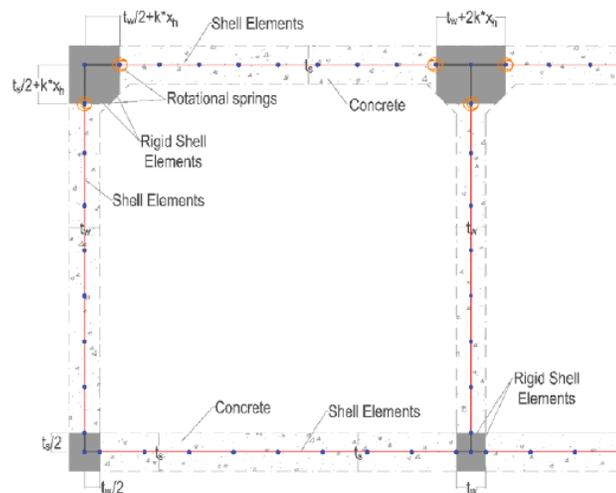
**Figure 17: 3D-Modeling of culverts using shell elements with rotational springs at wall/slab connections (Okeil et al., 2018)**
