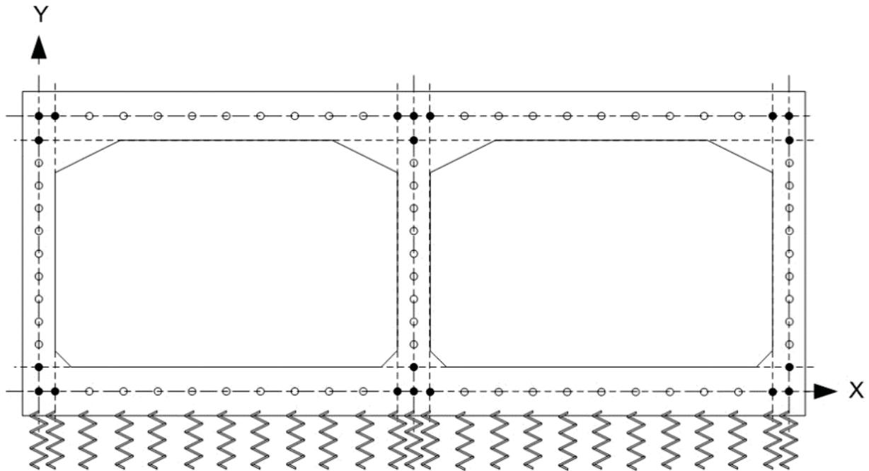
Figure 53: 2D Frame element model in Bridge Rating
