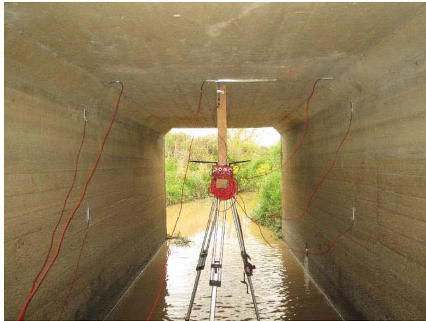
Figure 45: Photo showing the sensors installed in the exterior cell of the culvert
