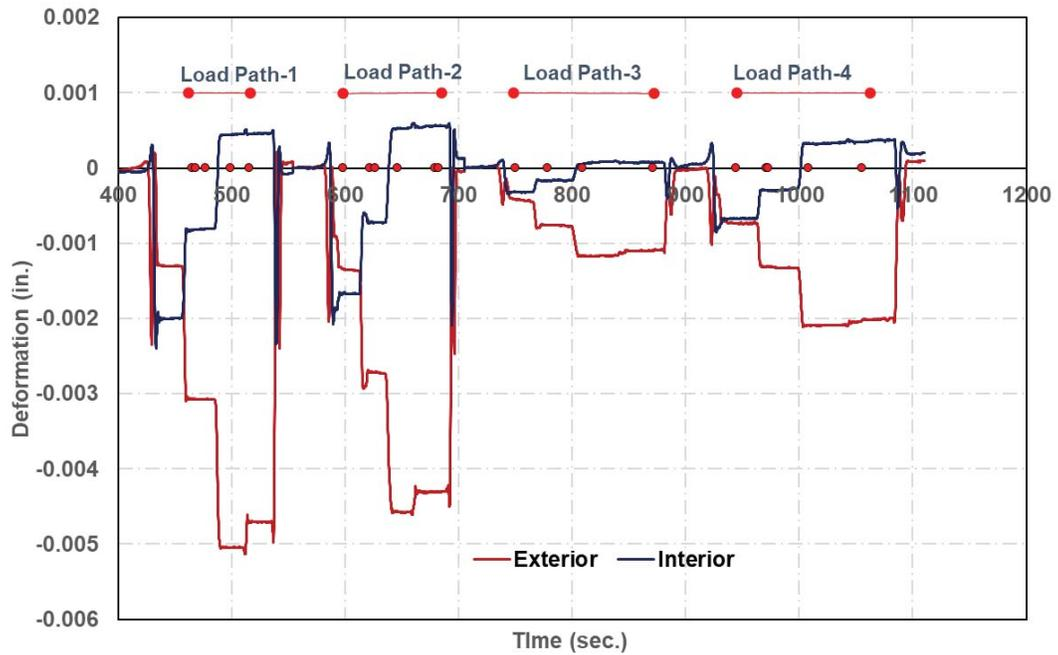
Vertical displacement at midspan of exterior and interior cells during loading of Culvert
