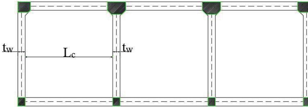
**Figure 57: Rigid parts that need be extracted from culvert span length**
