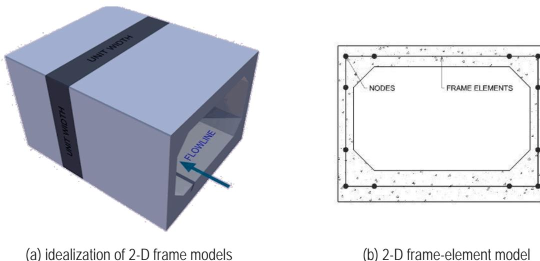
**Figure 14: Idealization of two-dimensional (2-D) frame-element structural model**
