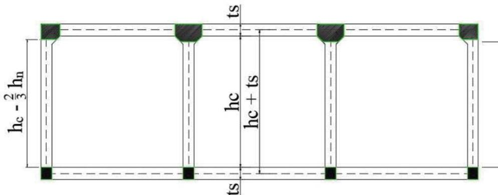
Figure 55: Rigid parts that need to be extracted from culvert height
