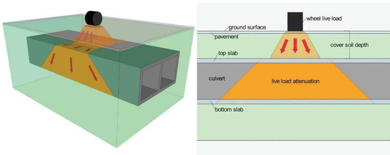
**Figure 9: Illustration of live load distribution for RC box culverts (Wood et al., 2016)**
