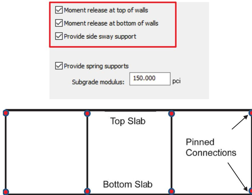
Figure 59: Applying the pinned connections to the 2D frame model in Bridge Rating software
