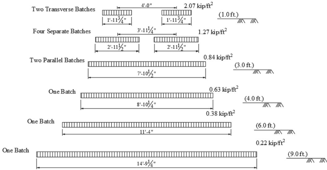
Live load distribution at the surface of the top slab in the direction parallel to span for 10 x 10 culverts
