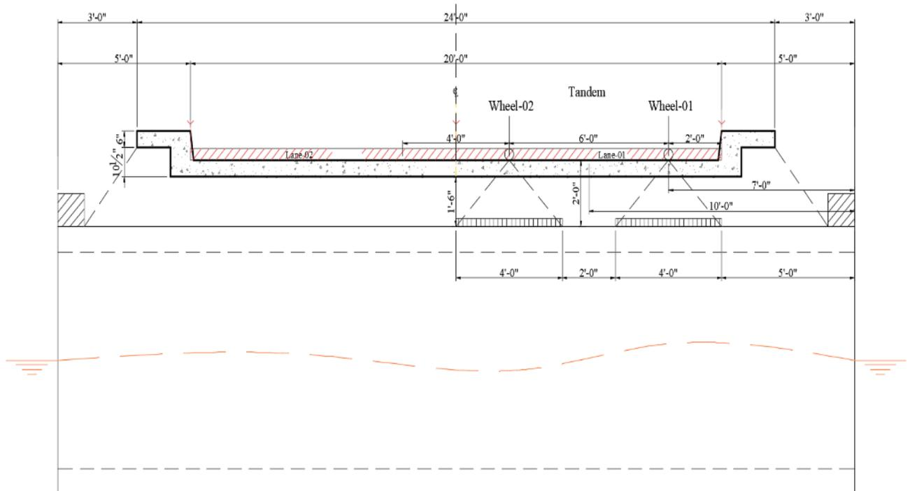
Live load distribution at the surface of the top slab in the direction perpendicular to the culvert span for fill height of 2.0 ft
