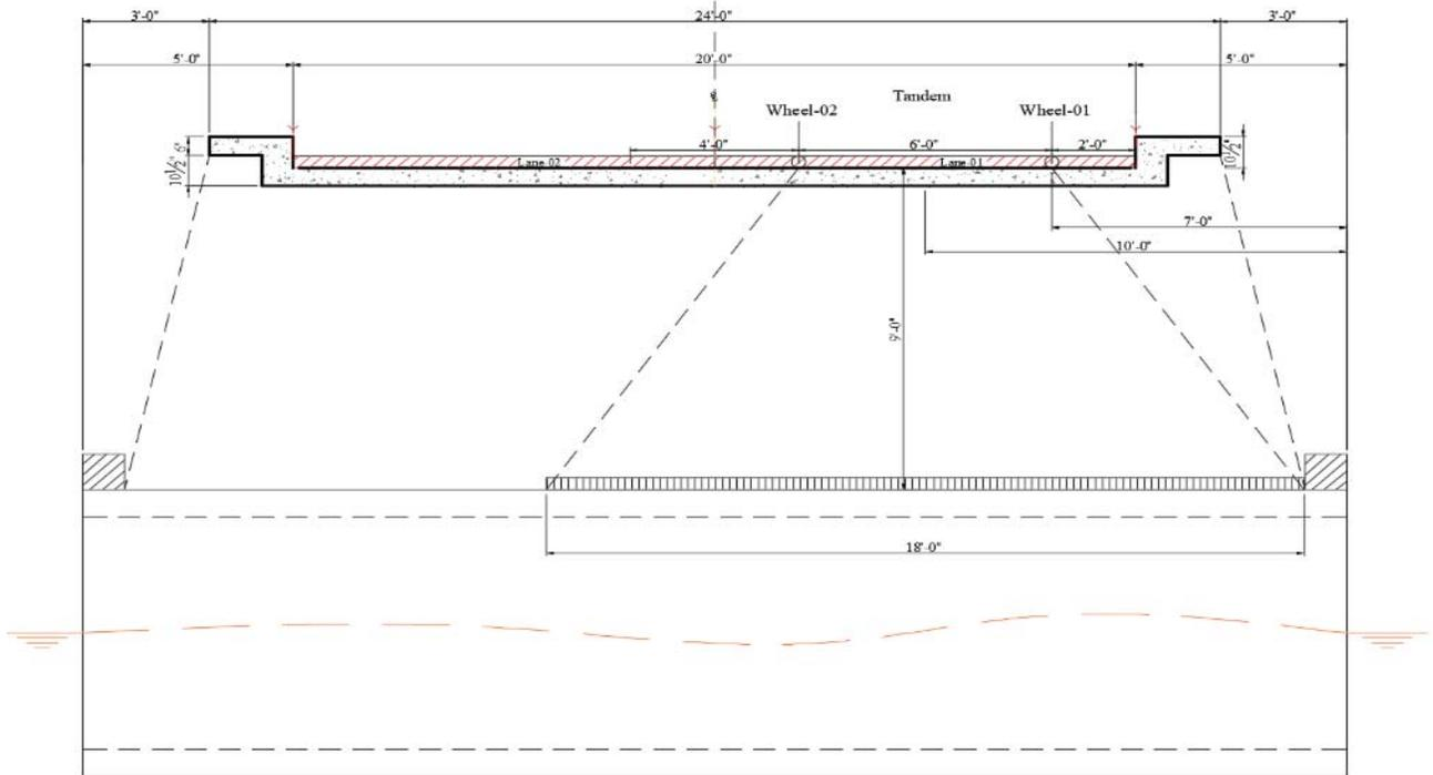
Live load distribution at the surface of the top slab in the direction perpendicular to the culvert span for fill height of 9.0 ft
