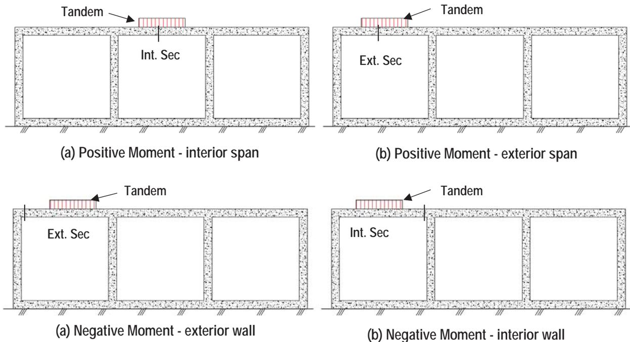
**Figure 30: Positioning of Tandem loading to produce maximum positive and negative moments at midspan and wall sections of the exterior and interior cells**
