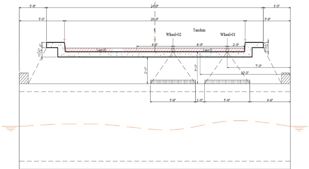
Live load distribution at the surface of the top slab in the direction perpendicular to the culvert span for fill height of 3.0 ft
