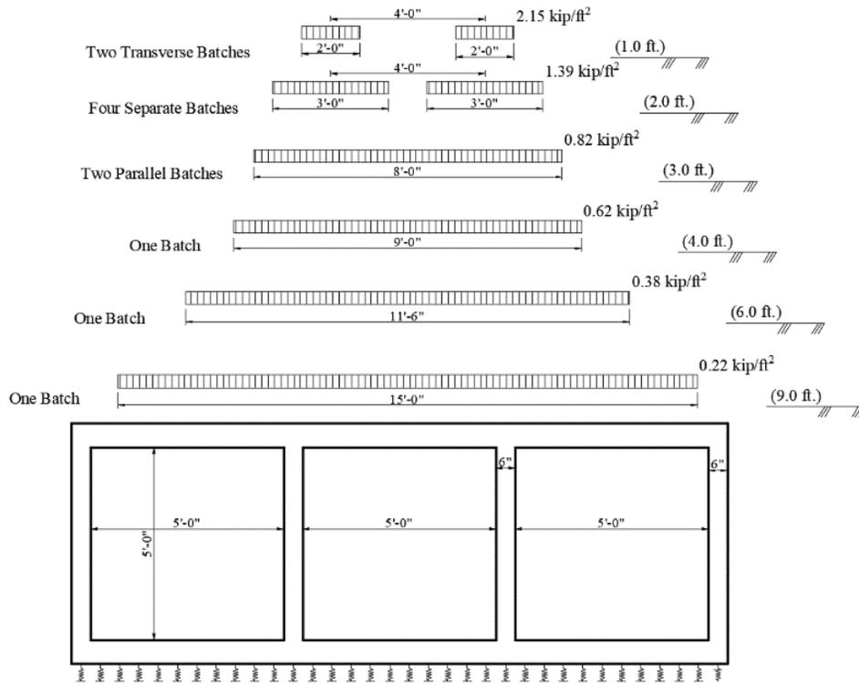
Live load distribution at the surface of the top slab in the direction parallel to span for 5 x 5 culverts
