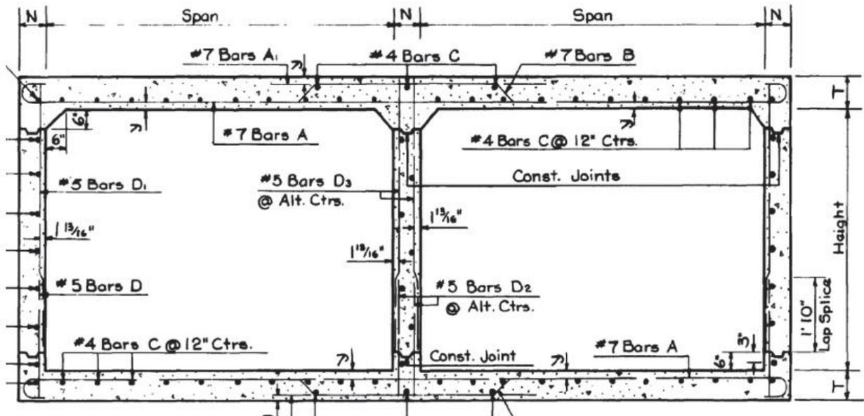
Figure 3: LADOTD standard reinforcement details of double-cell RC box culvert in Louisiana DOTD
