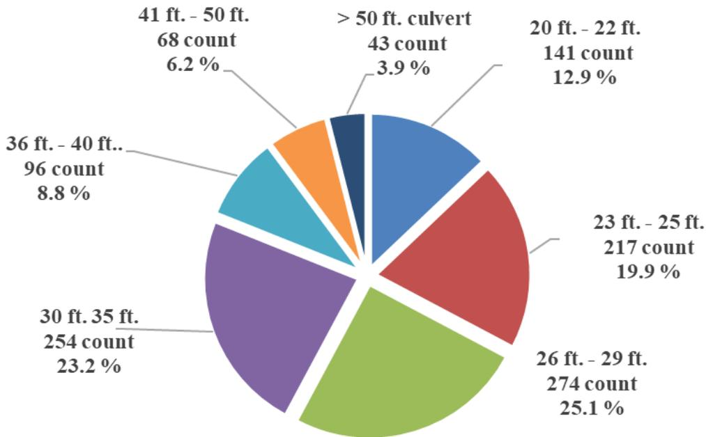
Figure 22: Classification based on the total width of the culvert
