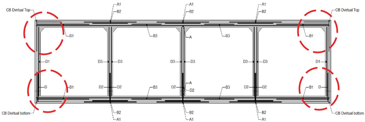
**Figure 61: Virtual reinforcements applied at the culvert four corners**
