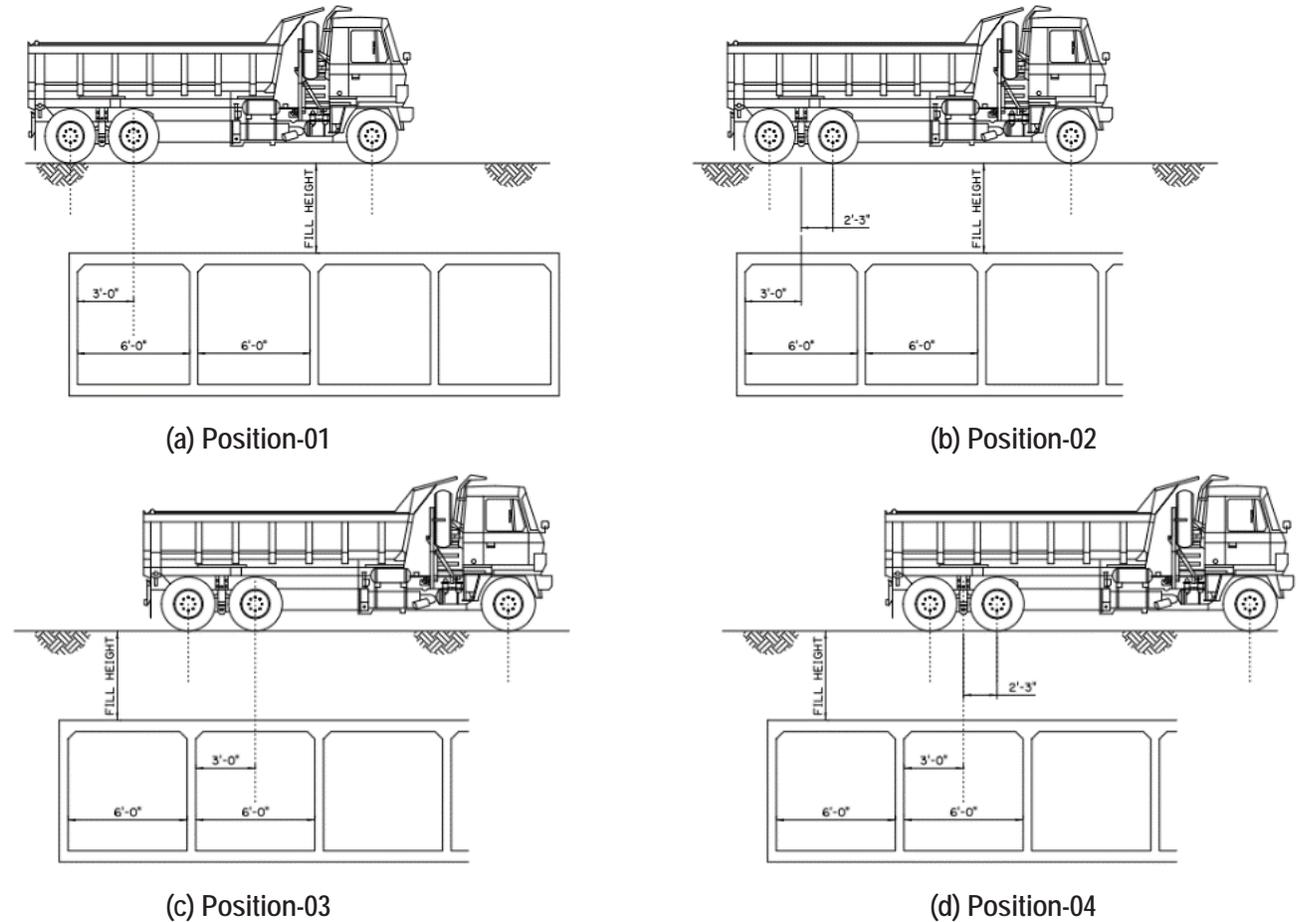
**Figure 47: Loading positions for each loading path**
