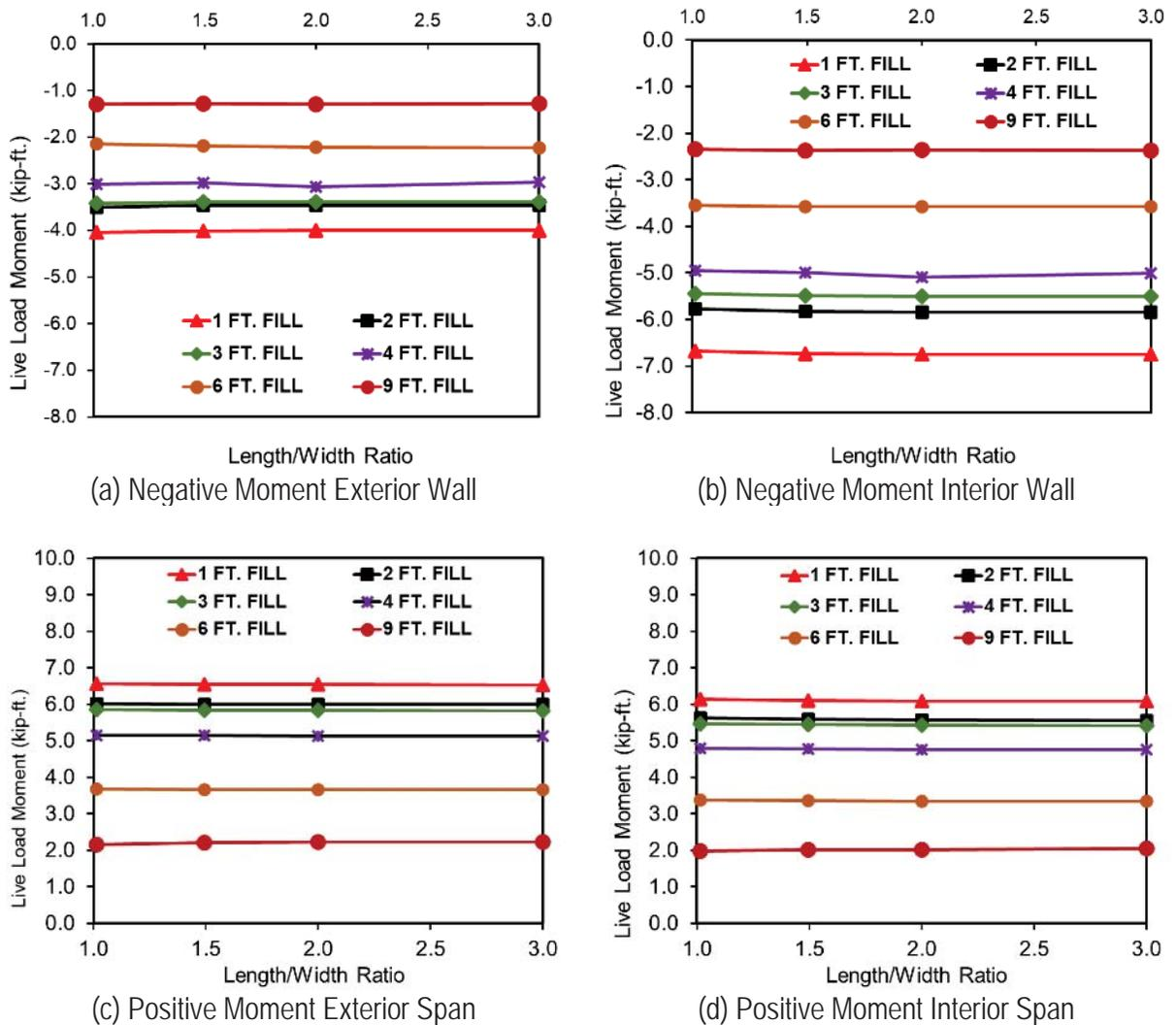
Figure 34: Live load moment from 3D models for 12X12 culverts
