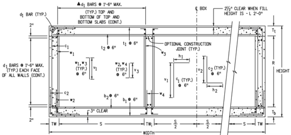
Figure 5: Colorado standard reinforcement details of Multi-cell RC box culvert in Colorado DOT
