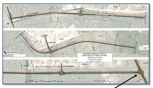
Project Relevance - Designed using the DOTD guidelines and software; includes similar design SOW (roundabouts, roadway widening, roadway realignment and reconstruction); project requires LADOTD review and approval
