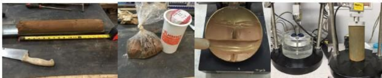
Laboratory Extrusion, Specimen Selection and Storage, Atterberg Limits, Consolidation, and Strength Testing
