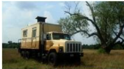
Fugro CPT Equipment (left to right): Truck-Mounted CPT, Total CPT equipment Track-Mounted CPT
