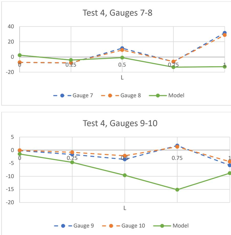
Figure 42 - Load Test 4 (Gauges 7-10) (: Axle 1 over Marked Points (Truck Centered) (M4C1)
