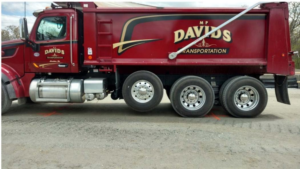
**Figure 26 – Wheel Loads/Configurations for Model 7-Candidate 1 (M7C1)**
