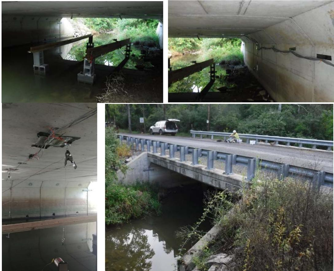
**Figure 1 – M1C1 Culvert Instrumentation**
