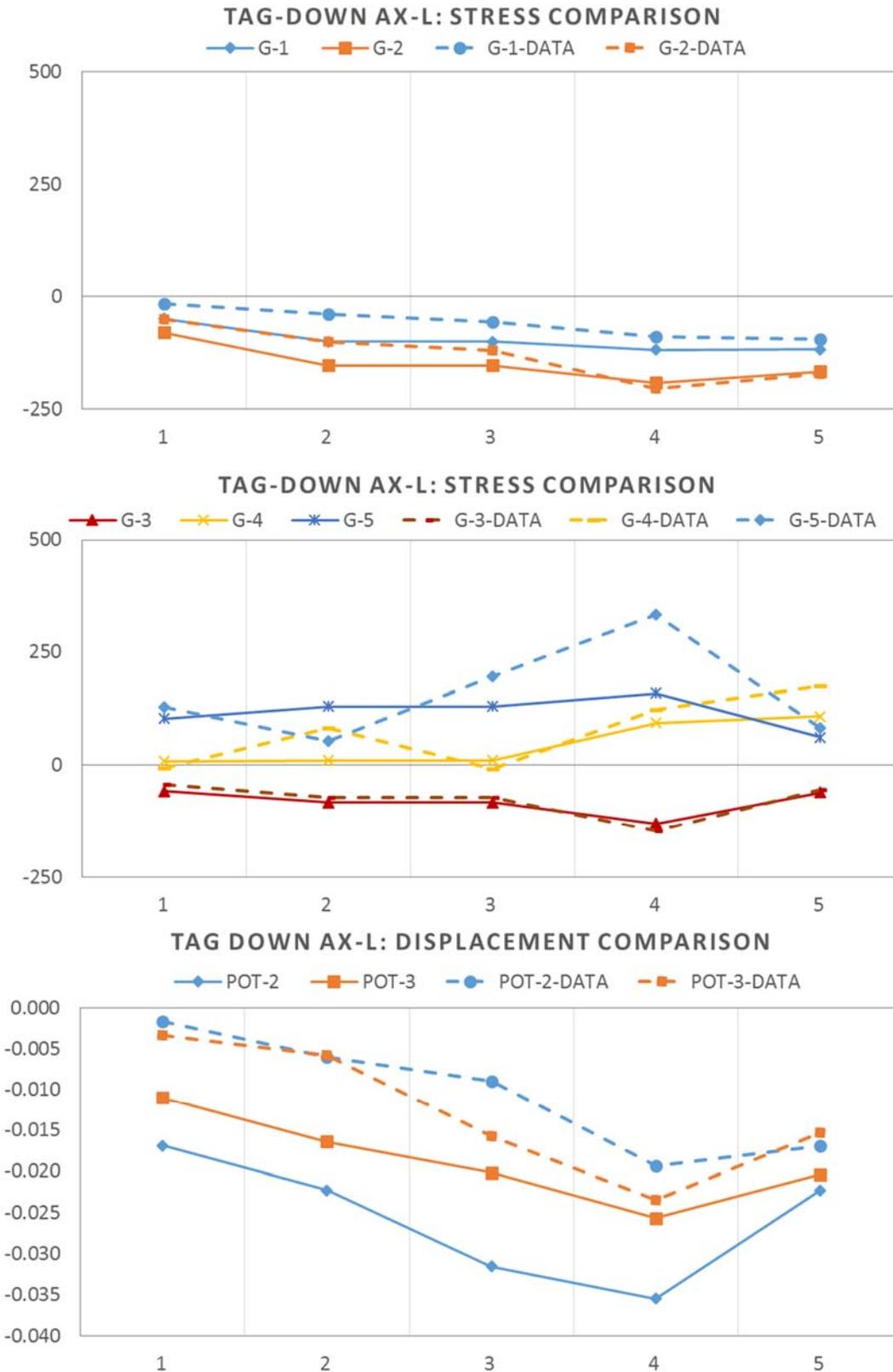
Figure 15 - Load Case D-L: Lift Axle Down and Lift Axle Left Wheel over Marked Points (M1C1)
