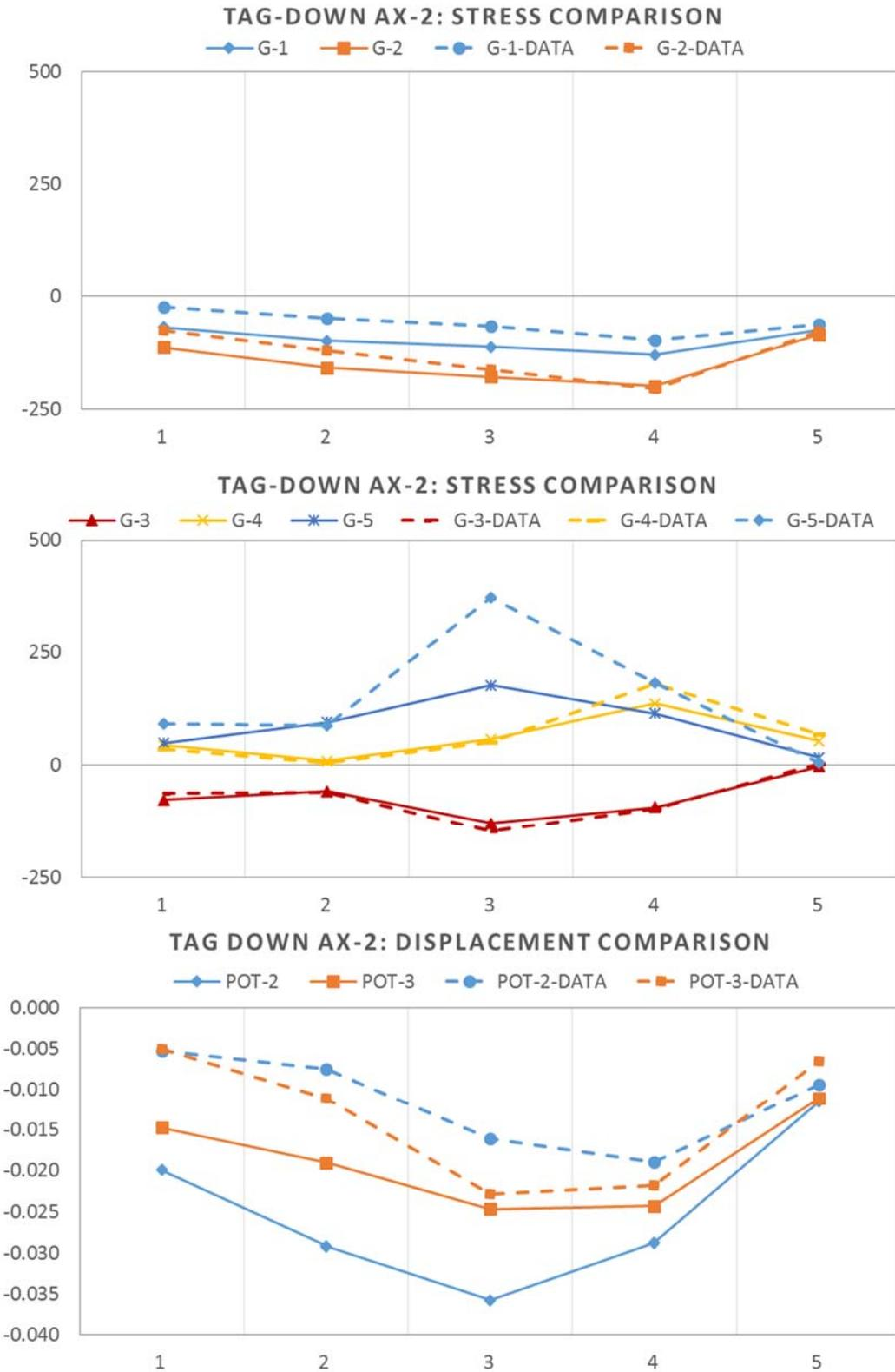
Figure 13 - Load Case D-2: Lift Axle Down and Axle 2 Left Wheel over Marked Points (M1C1)
