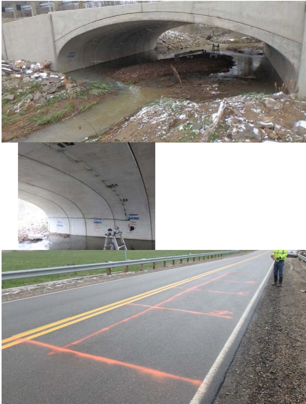
**Figure 16 – M4C1 Culvert Instrumentation/ Load Line**
