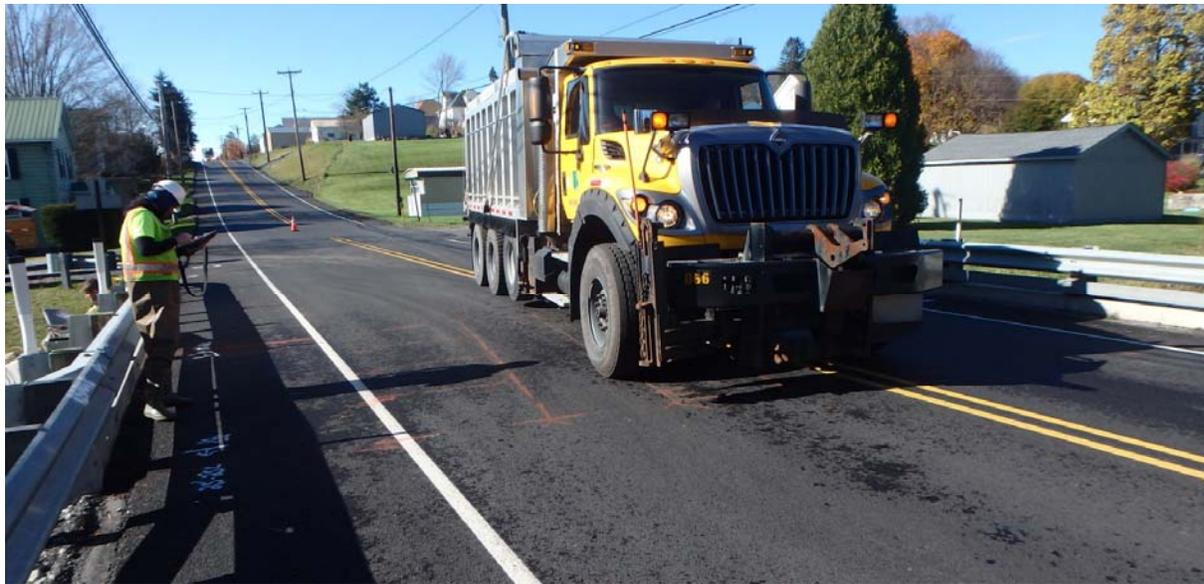
**Figure 13 – M3C1 Load Testing**
