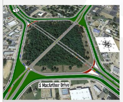
Figure: VISSIM Animation of Grade Separated Intersection Concept
