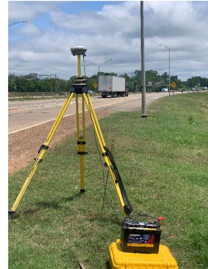
In order to establish the baseline, we will set an autonomous base point near the bridge. Then using RTK, we will tie surface features along the bridge and any monuments found along the baseline. Once the baseline is established relative to the base point, RTK can be used to determine the exact location of the predetermined offsets along the cross-sections.
