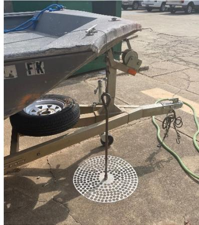
In order to determine the exact locations of the required soundings, the transducer for the fathometer is mounted to the back of our boat with a GPS receiver mounted directly above the transducer. The transducer mount maintains a constant draft for the duration of the survey.
