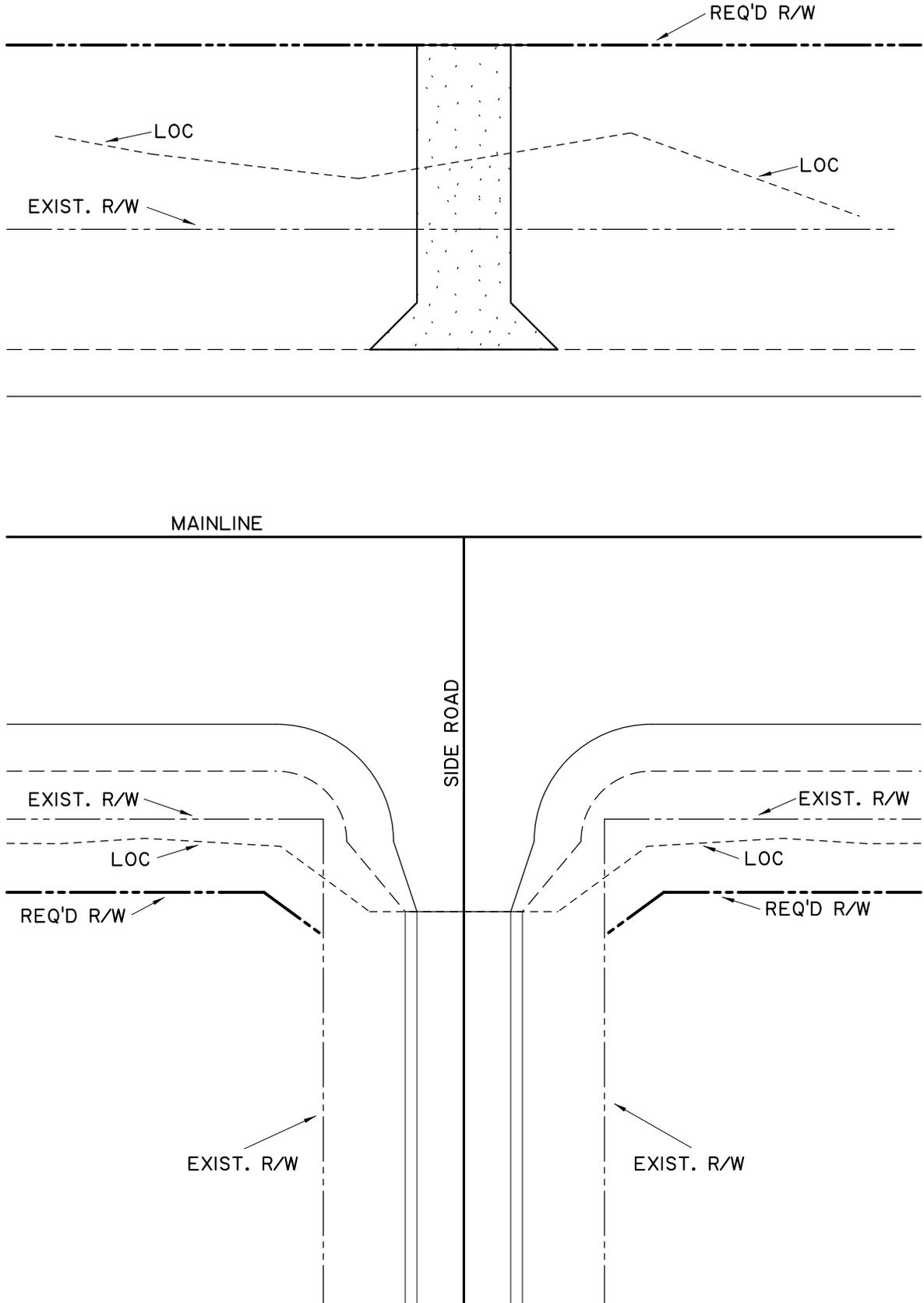
FIGURE 8-21: LIMITS OF CONSTRUCTION IN PLAN VIEW
