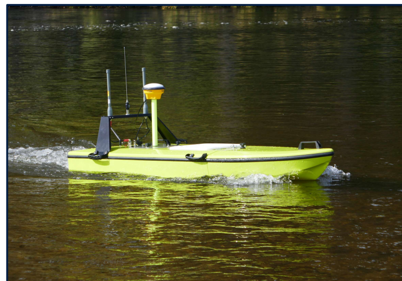
Our Uncrewed CEE-USV Collecting Single Beam Data
