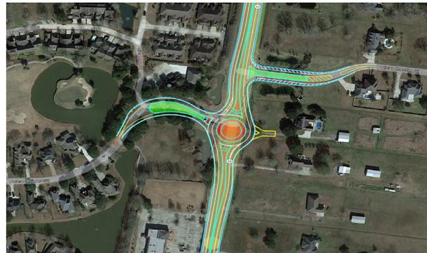
Figure 1 - LA 44 and Pelican Point Roundabout Potential Layout
