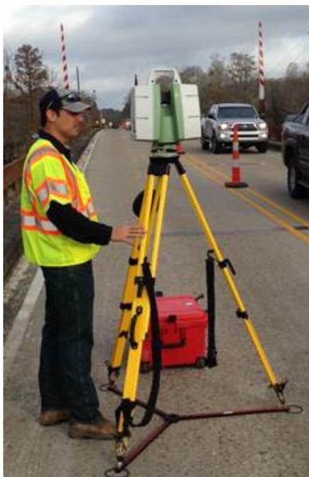
*Figure 2: Photograph of Leica ScanStation C10*
