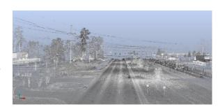
practices/procedures. All deliverables were in LADOTD required formats. **3D Terrestrial Scanning** was used in conjunction with traditional means and methods to complete this project.
