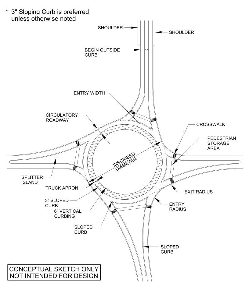
Figure 6-09 Roundabout Parts
