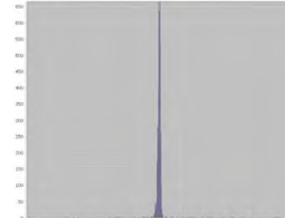
Figure 8. Histogram distribution of elevation difference between Figure 2 SuperNova data and mobile lidar control surface
