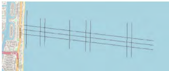
Figure 2. Bathymetric boresight flight pattern near Fort Lauderdale, FL
