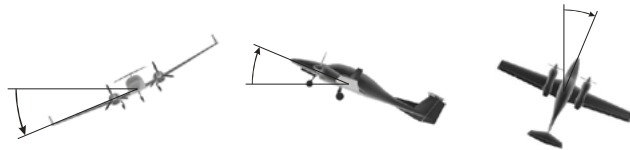
Definition of the axis of the aircraft-own coordinate system
