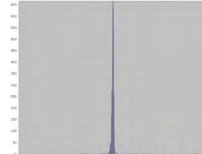
Figure 8. Histogram distribution of elevation difference between Flight 3 SuperNova data and mobile lidar control surface
