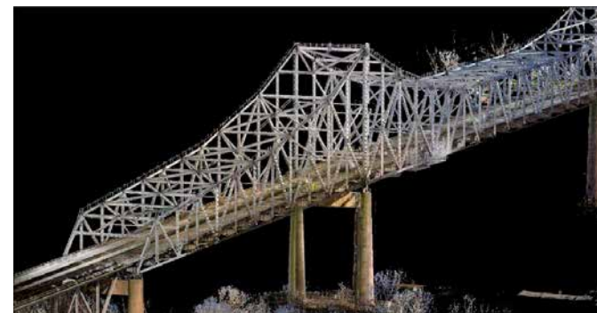
Laser Scan Survey of Sunshine Bridge in Donaldsonville, LA
