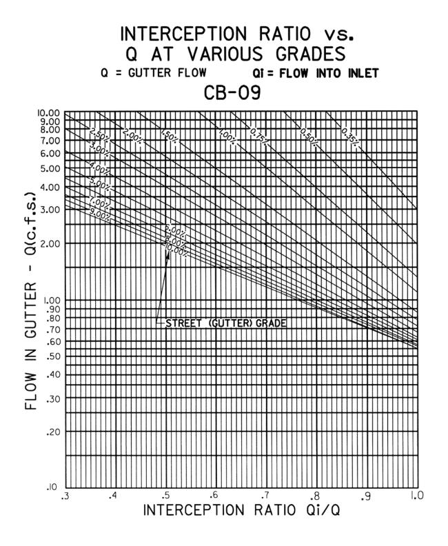
Figure 8-A.8-4 CB-09 Inlet Capacity Curve on a Grade (Inside of Pavement)
