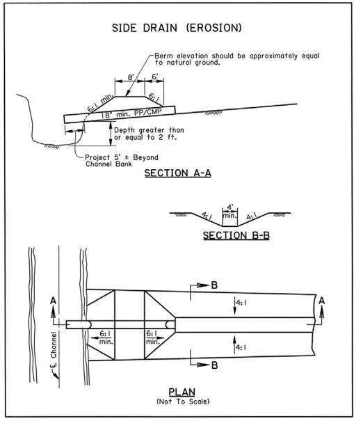
Figure 4.8-1 Channel Block - Side Drain (Erosion) Example
