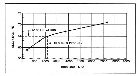
Figure 4-A.5-1(b) Stage–Discharge Curve for Example Problem 4-A.5.1
