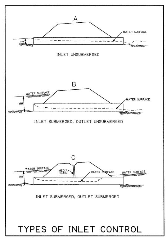
Figure 6-A.6-1 Examples of Inlet Control
