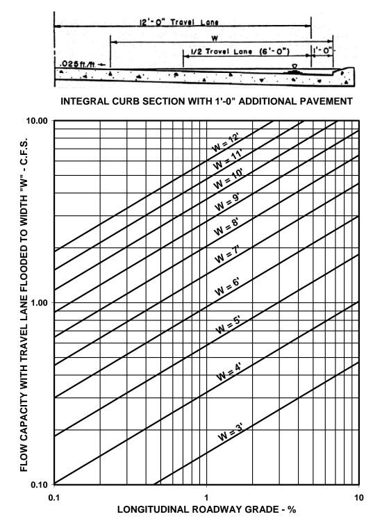
Figure 8-A.7-1 Gutter Capacities For Uniform Cross Slope of 0.025 ft/ft
