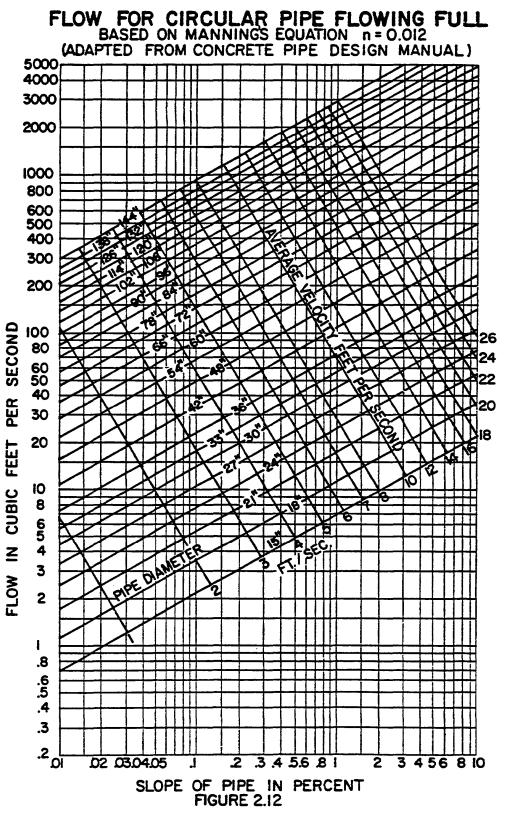
Figure 8-B.6-1 Flow for Circular Pipe Flowing Full
