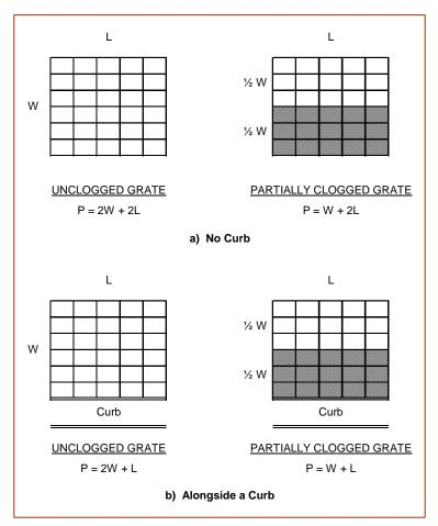
Figure 8-A.3-1 Perimeter (Weir Crest Length) of Grate Inlets
