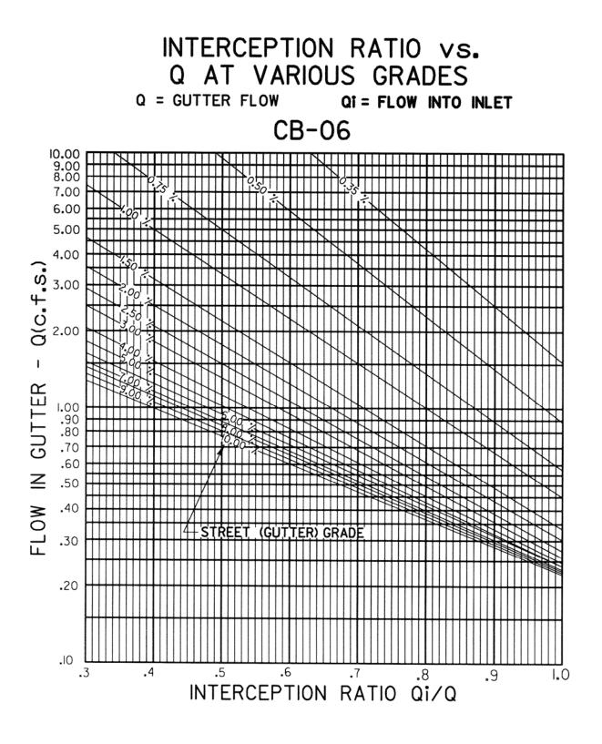
Figure 8-A.8-1 CB-06 Inlet Capacity Curve on a Grade (Inside of Pavement)
