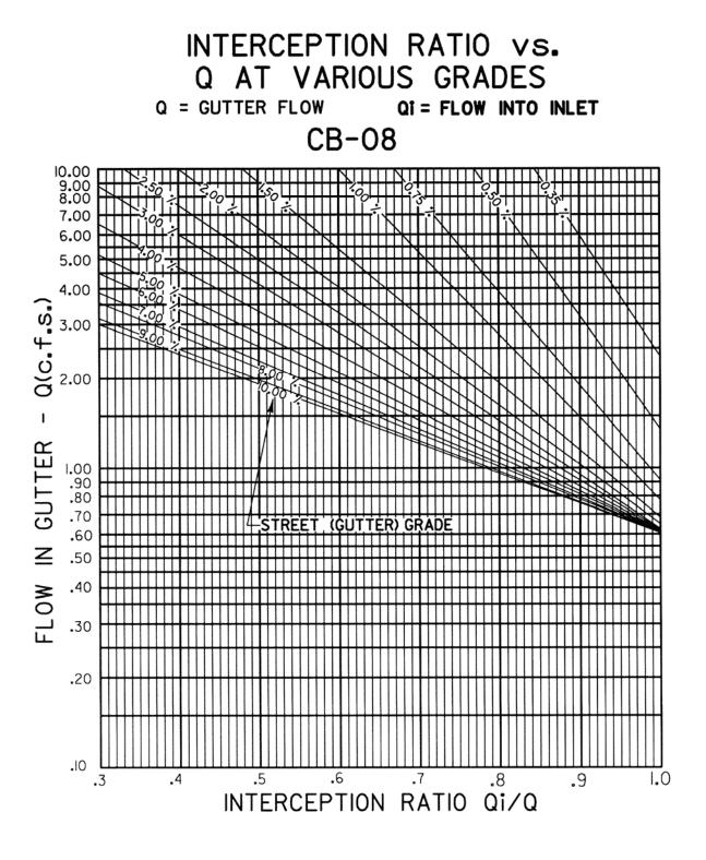
Figure 8-A.8-3 CB-08 Inlet Capacity Curve on a Grade (Inside of Pavement)
