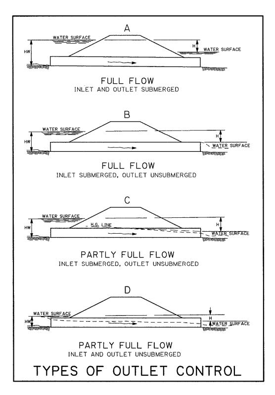
Figure 6-A.7-1 Examples of Outlet Control
