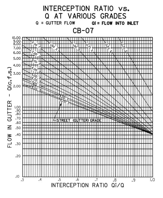
Figure 8-A.8-2 CB-07 Inlet Capacity Curve on a Grade (Inside of Pavement)
