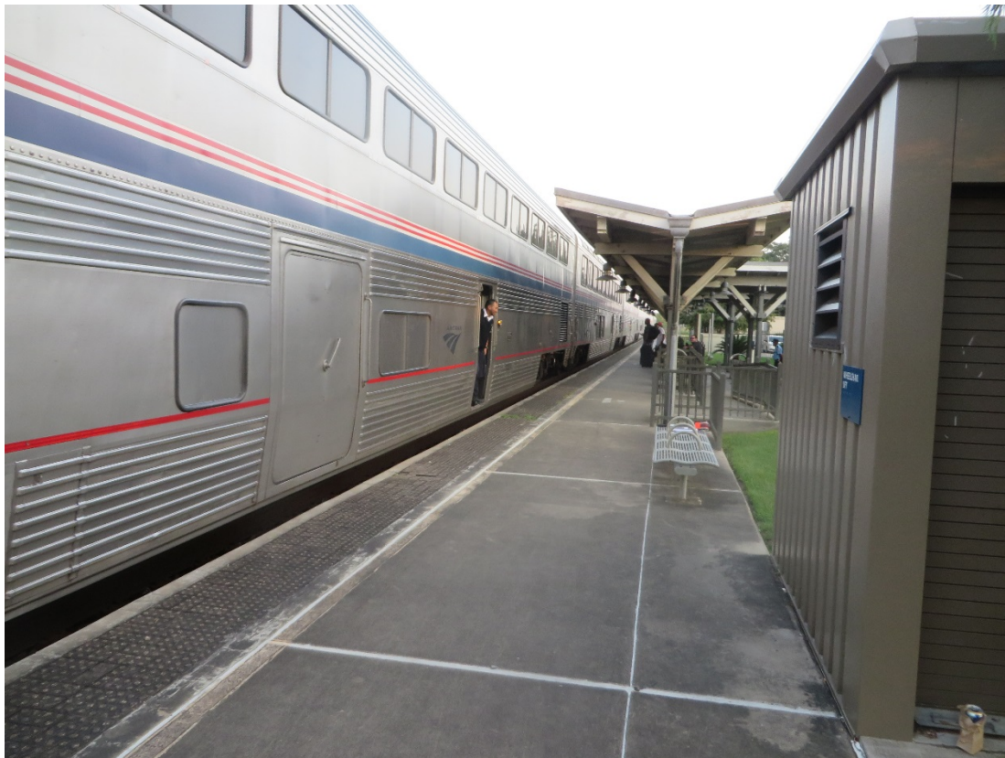
Figure C-7. Train stopped at platform depicting platform height relative to train (looking southwest).
