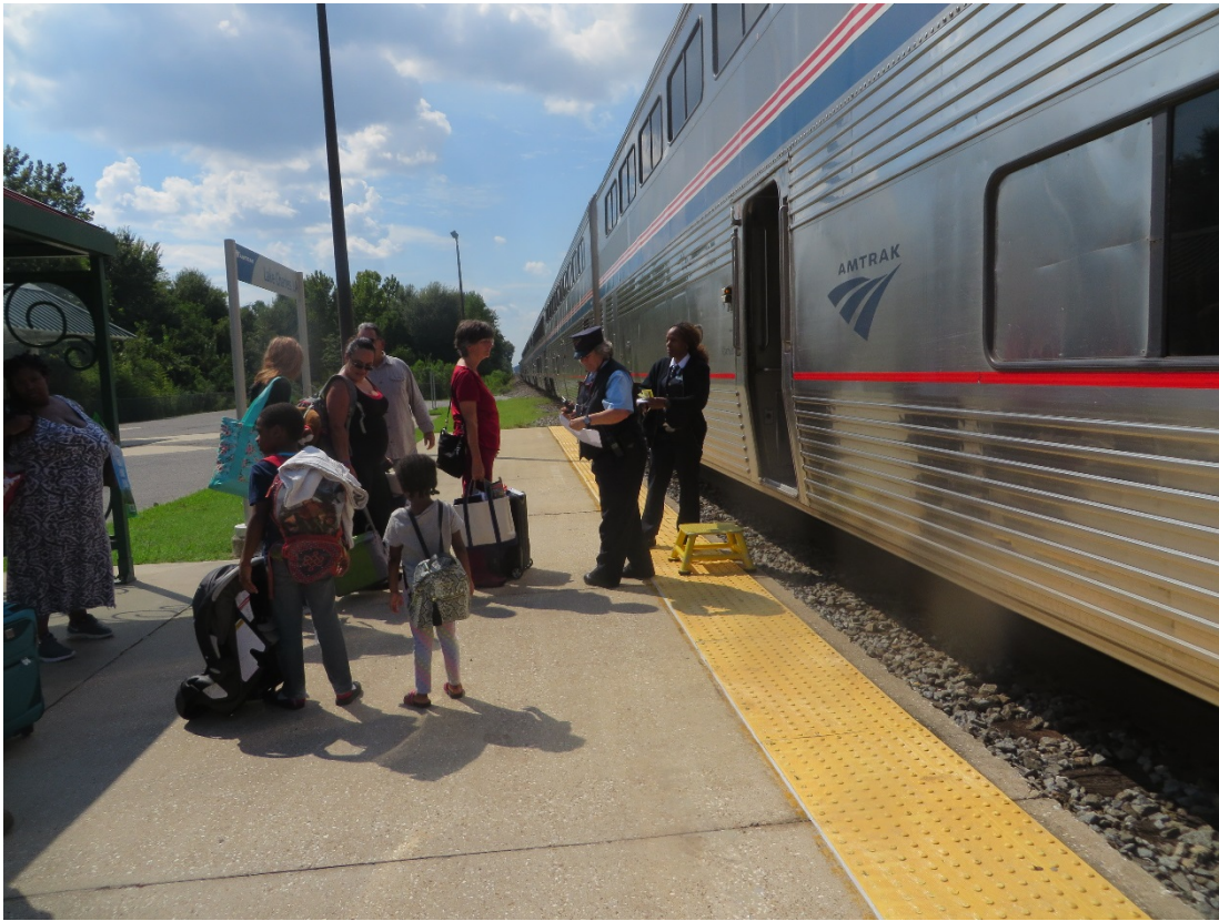
Figure B-3. Level boarding does not exist; step stool used to assist passengers board the train.
