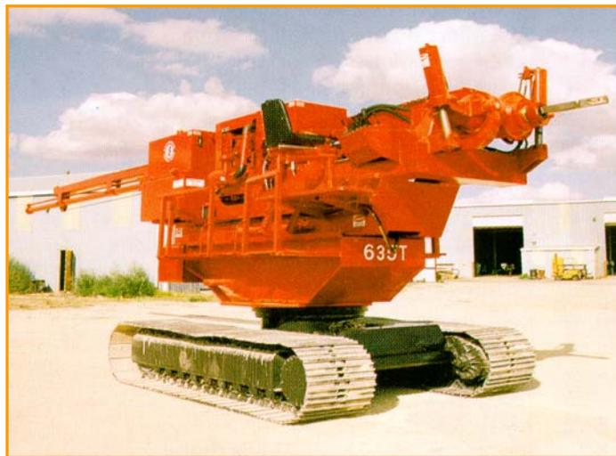
**Figure A-22: Two types of Drilled Shaft Foundation Construction Equipment.**
