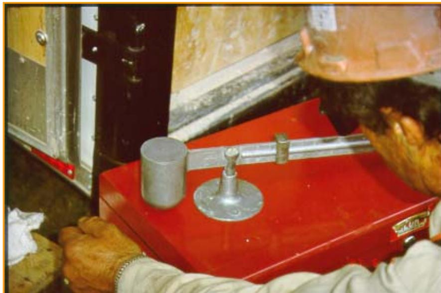
**Figure A-15: Testing the density of the Bentonite Slurry**
