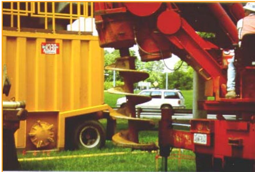
**Figure A-2: Drilled Shaft Soil Auger or Flight Auger**
