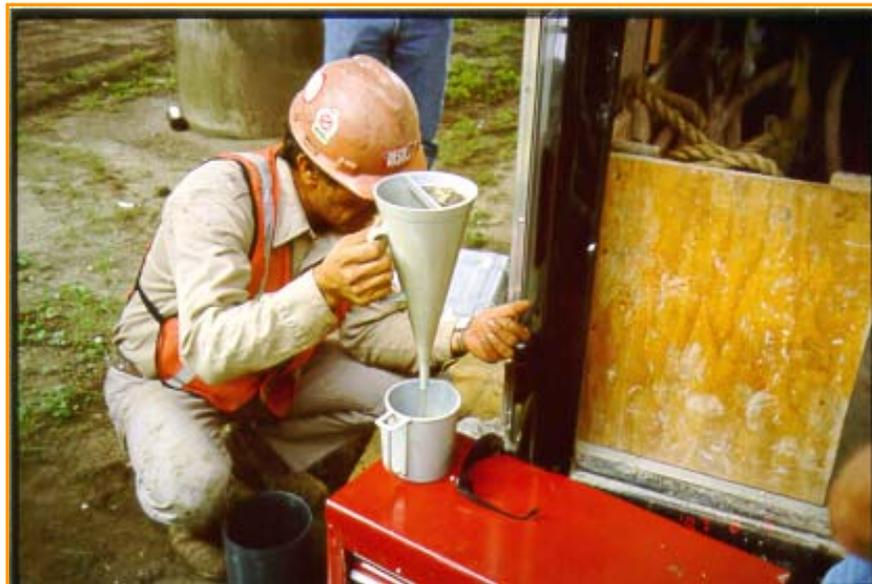
**Figure A-13: Marsh Funnel Viscosity Test**
