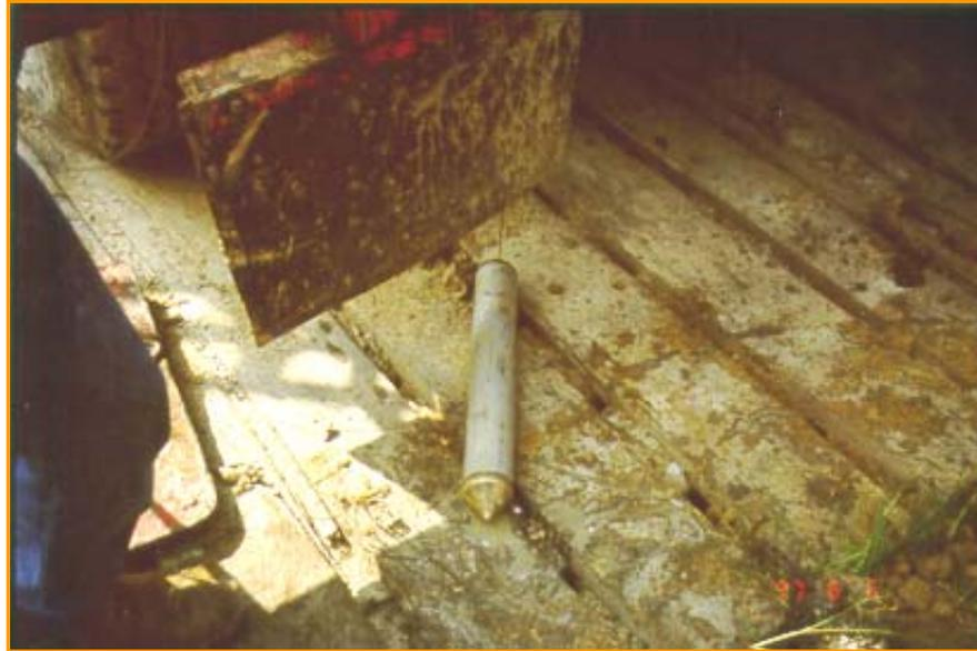
**Figure A-12: Cone Slurry Density sampler.**
