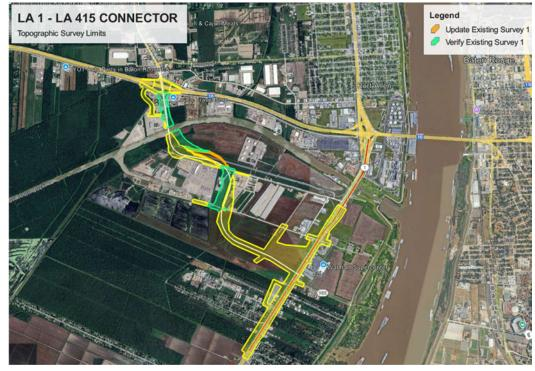
traffic segments of LA 1, Interstate 10 ramps, and LA 415. The data was processed through Trimble Business Center, with data extraction performed through TopoDot. The survey is being conducted according to the Louisiana Department of Transportation and Development Location and Survey Manual. The deliverables will be provided in accordance with the LADOTD guidelines for electronic deliverables.
