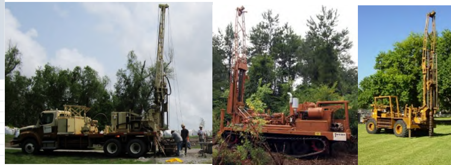
Fugro Drilling Equipment (left to right): Summary of available Drilling Rigs, Truck, Track, ATV Rigs
