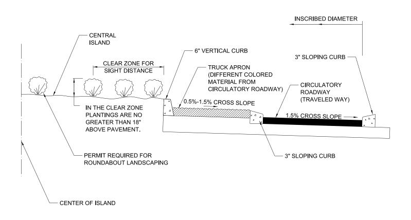
Figure 6-10 Central Island Cross Section
