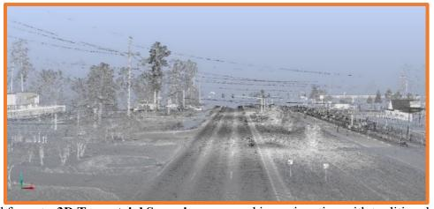
standard practices/procedures. All deliverables were in LADOTD required formats. **3D Terrestrial Scanning** was used in conjunction with traditional means and methods to complete this project.
