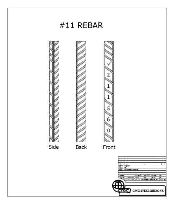
Products: Billet-Steel Deformed Bar, Grade 60 (#4, #5, #6, #7, #8, #9, #10 and #11)
