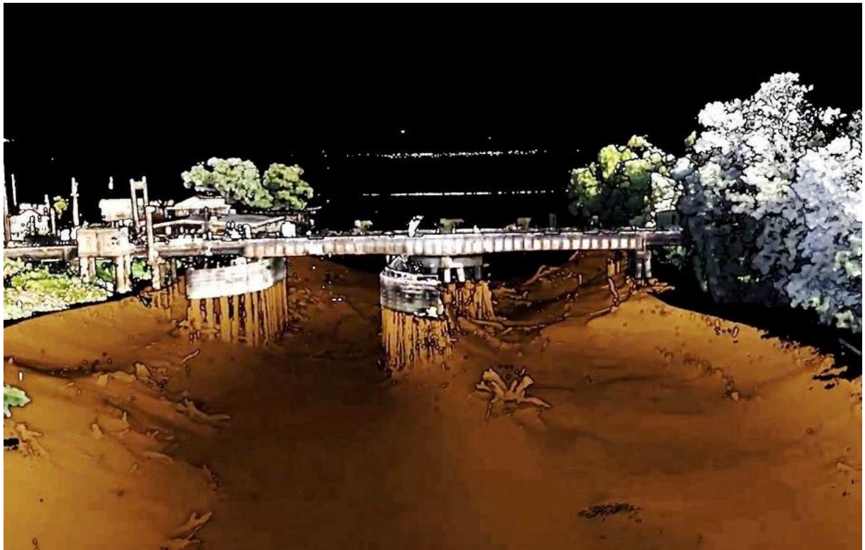
Port Vincent Bridge Scan and Bathymetry Integrated
