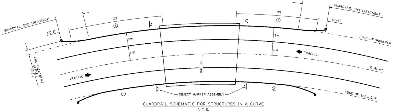
FORMULA FOR COMPUTING GUARDRAILS LENGTH OF NEED (X) IN A CURVE
