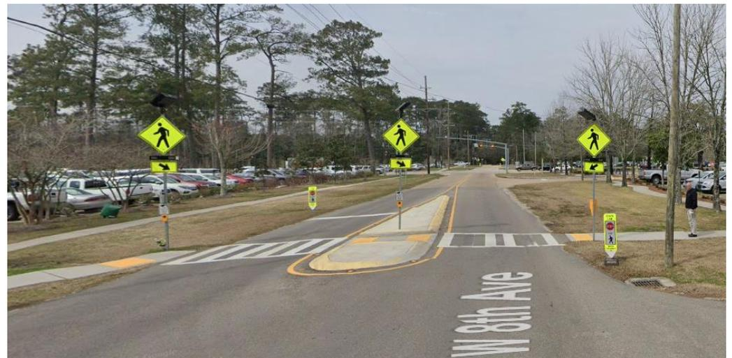
Rectangular Rapid Flashing Beacon assembly, known as the RRFb, is pedestrian actuated crosswalk beacon that flashes to alert drivers when someone is crossing. Shown here at W. 8<sup>th</sup> Ave in Covington.
