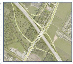
Interchange (DDI), an innovative approach in interchange design. The Pecue Lane DDI provides a higher level of operational efficiency and is a safer alternative to a conventional diamond interchange. It will consist of three thru lanes in each direction with raised medians and sub-surface drainage.
