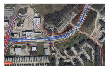
The final preferred alternative was evaluated as part of the final analysis. ATG compared the proposed alternatives with the existing geometry to identify a reduction in conflict points as part of the safety analysis. HCS was used to evaluate the ramps, basic segments, merge and diverge areas, and weave locations for the proposed alternatives.
