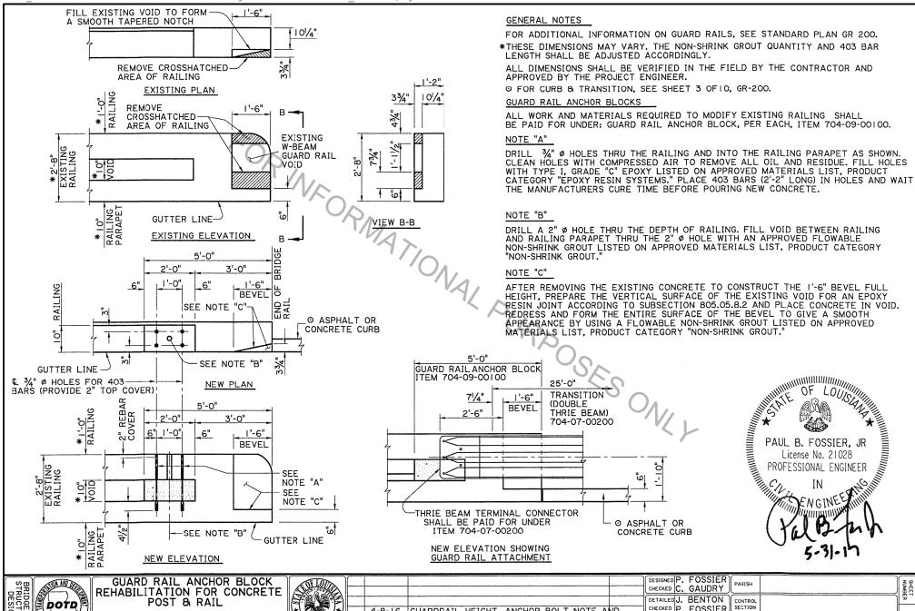
GUARDRAIL HEIGHT, ANCHOR BOLT NOTE AND
