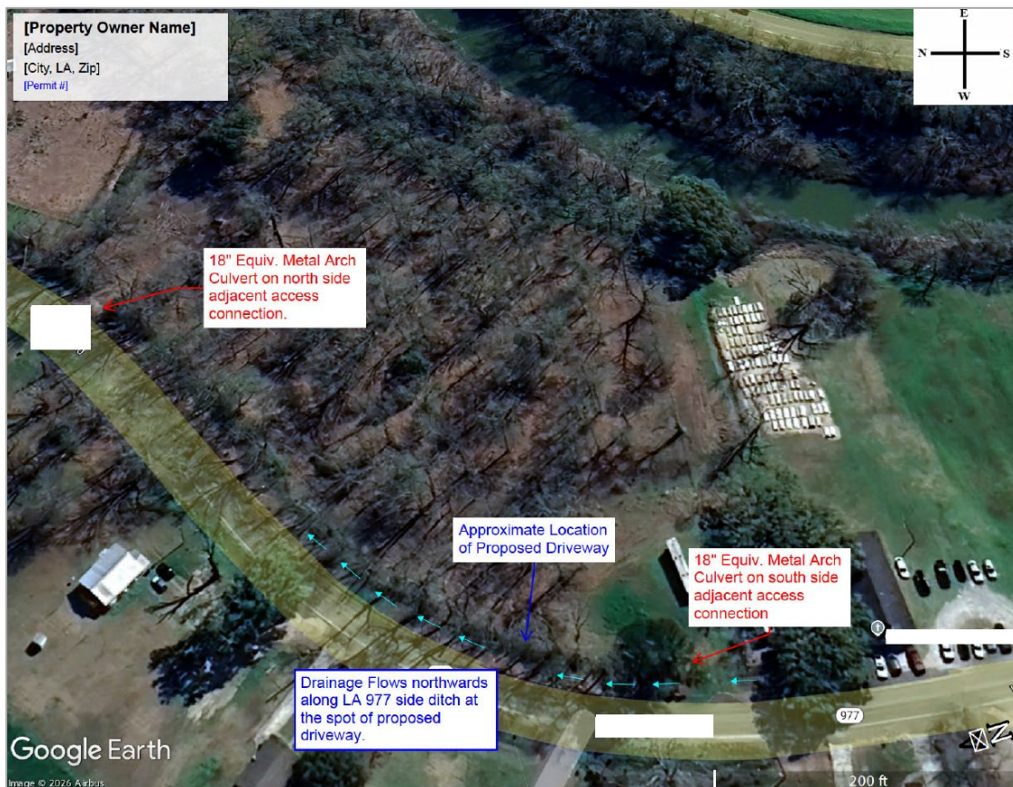
Figure 1.8e: Google Earth Aerial View — Residential Access Connection Permit Example (SANITIZED). Shows the project site with the approximate location of the proposed driveway, existing adjacent culverts on the north and south sides (18-in. equivalent metal arch), and drainage flow direction (northward along the [State Highway] side ditch). Prepared by the Water Resources Technician during the site assessment (Step 3).
