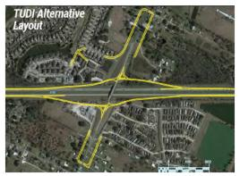
options like this one where the ramp terminal signals are relatively close to each other, signal timing and phasing will need to be optimized to promote smooth operations, and sight lines will need to be checked to ensure adequate stopping sight distance is provided at the bridge. Effects of the signalized ramp terminals on nearby intersections, especially the intersection of LA 74 at LA 73 (approximately 2700 feet west), will also need to be analyzed.
