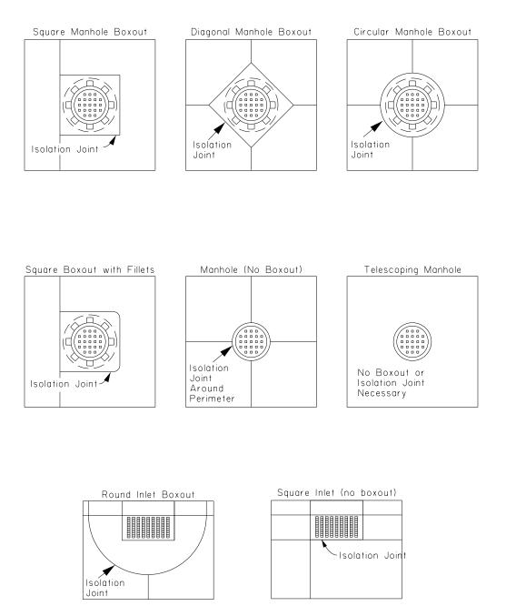
Notes: I. Isolation Joints Should be at least 1/2" Wide and Filled With a Compressible Material
